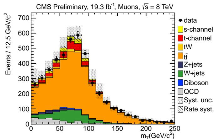
FIGURE III.1: Transverse mass of the  $W$  boson in 2J2T category for the muon channel.
