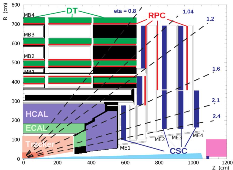
FIGURE II.9: The muon system of the CMS detector.
