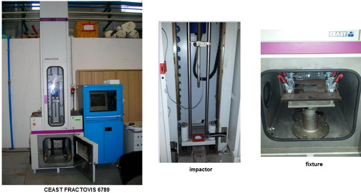
**Figure 73: impact machine and fixture**
