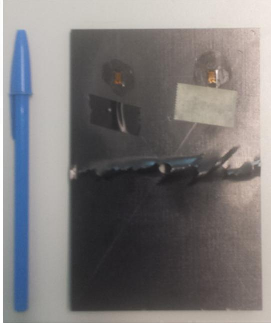
Figure 79: 28-ply laminate – open hole CAI coupon after compression test
