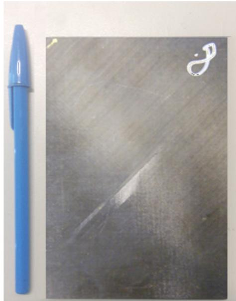
Figure 77: 28-ply laminate – impact test at 50 joule
