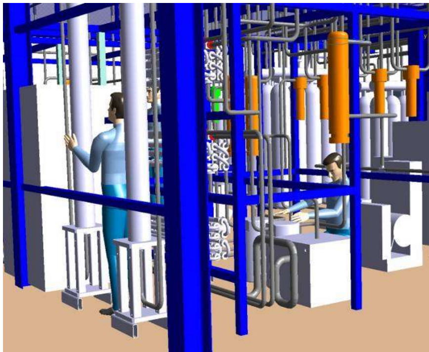
Figure 4.10 Maintenance walkways for Q 2 O adsorbers and oxidizing bed
