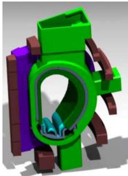
Figure 3.31 - DEMO divertor vertical upper port
