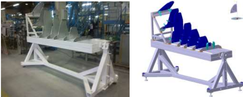
Figure 6.5 Physical model VS digital model of the dorsal fairing jig (Courtesy of LAER Aeronautical Manufacturing)
