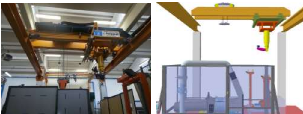
Figure 5.25 Real model VS Virtual Model of IFMIF test platform (Courtesy of ENEA Brasimone Research Centre)
