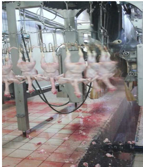
Figure 20. Feathers removal by means of mechanical pluckers.
