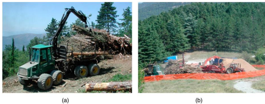
Figure 29. Loose residue chain: (a) forwarding loose residue from the yarder pad and (b) chipping them at the roadside landing.
