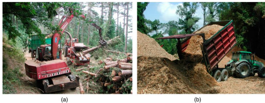
Figure 28. Chipped residue chain: (a) chipping at the yarder pad and (b) dumping the chips at the roadside landing
