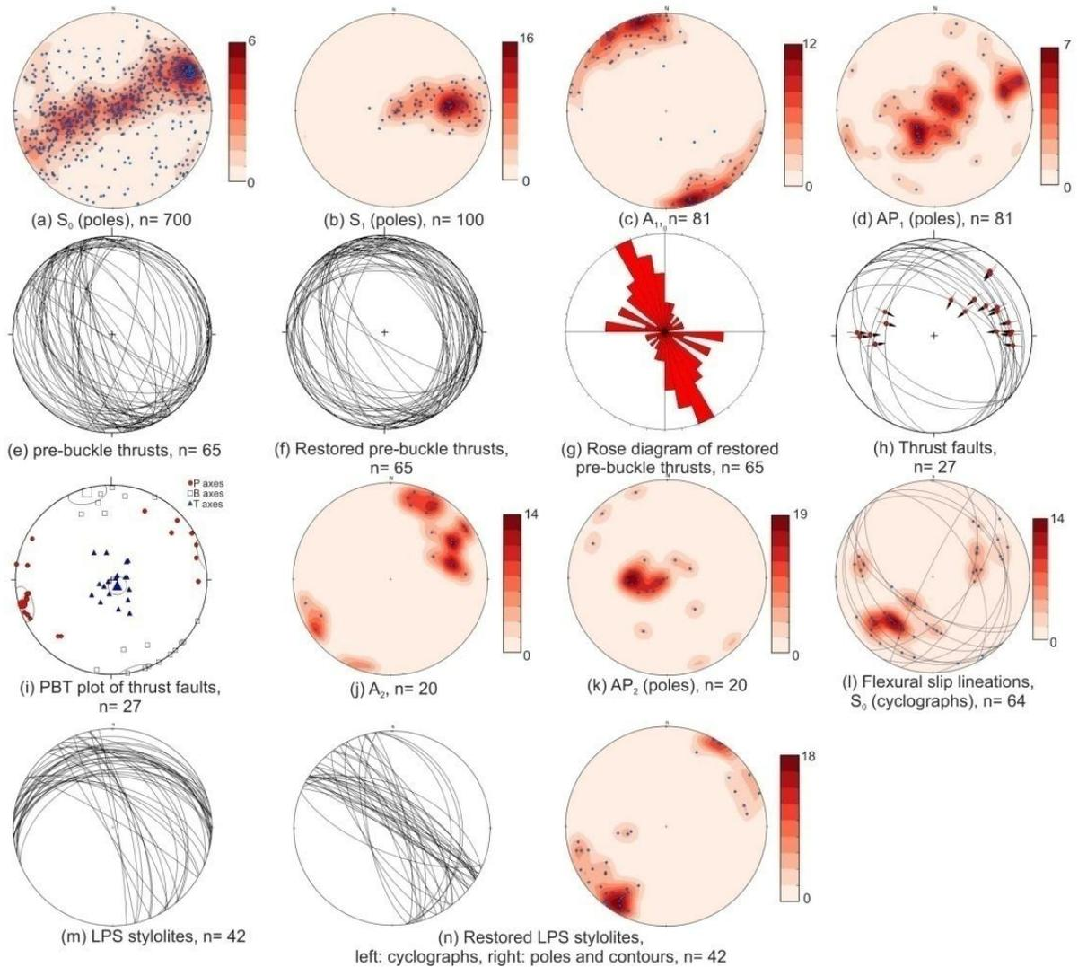
Fig. 47- Stereographic projections (equiareal net, lower hemisphere), rose diagram, contour and PBT plots (Angelier and Mechler, 1977; Reiter and Acs, 1996-2003) of the analyzed orogenic structures. PBT plot of thrust faults: P (254/05) R = 82%, B (345/06) R = 79%, T (133/83) R = 91%.
