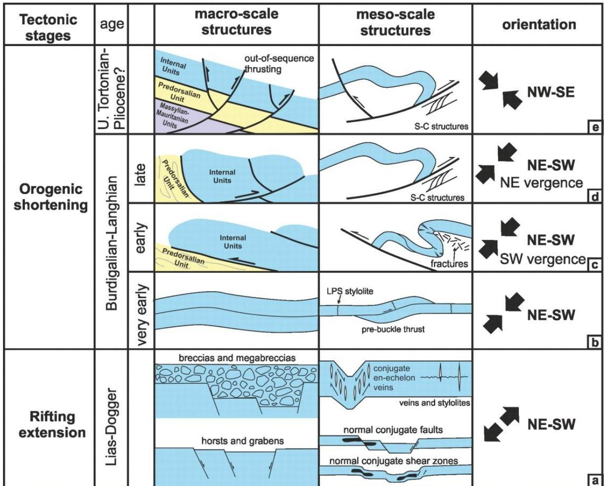
Fig. 49- Cartoon showing deformation structures at macro- and meso-scale and related deformation orientations and ages.
