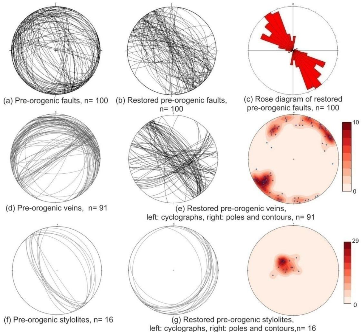
Fig. 44- Stereographic projections (equal-areal net, lower hemisphere), rose diagrams and contour plots of the analyzed pre-orogenic structures.
