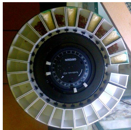
Figure 2.3 Representation of the automatic feeder and probiotic administration
