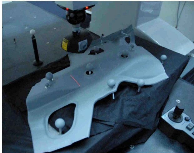
Figure 3: Acquisition phase with CMM laser scanner to generate the reference 3D model.
