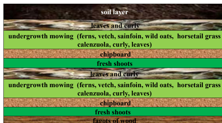
Fig. 1. Order and composition of layers in the biodegradation bin
