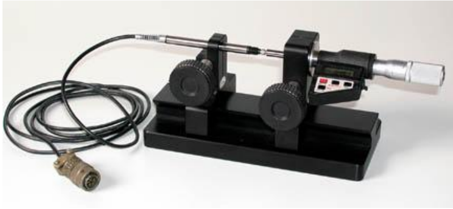
Figure 3.12. Typical LVDT calibration device
