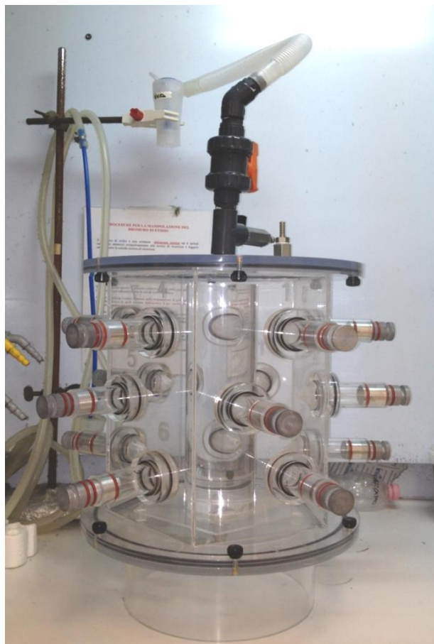
Figure 2.1. Apparatus used for administration of aerosolised NaHS.
