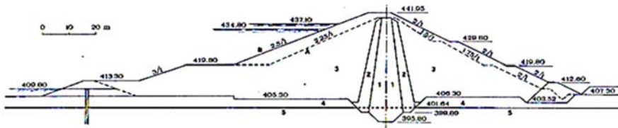
Figure 5.1 Cross Section of the Conza dam: A) original section, B) final section. Different zones: 1) core, 2) filters, 3) shell, 4) alluvial material, 5) foundation clay (Brigante, 2010).
