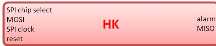
**Figure 4.13:** Input and output lines of the interface between CLK-Board and HK. All the lines are LVDS lines.
