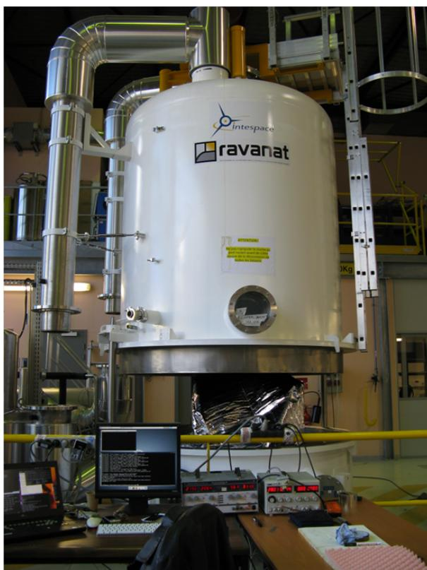
**Figure 5.7:** Figure 36 The CNES Simeon environment chamber.
