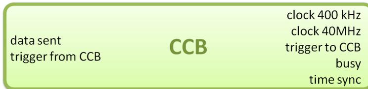
**Figure 4.15:** Input and output lines of the interface between CLK-Board and CCB. All the lines are LVDS lines, in order to maximize signal integrity.
