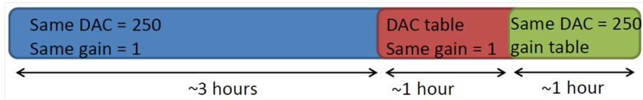
**Figure 7.3:** The data acquisition mode used during the flight.
