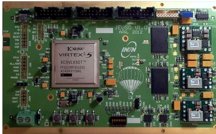
**Figure 4.8:** The CLK-Board of EUSO pathfinder. Apart from the FPGA, the board hosts the components to provide FPGA power and connections.
