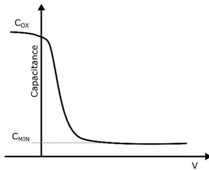
**Figure 2.7:** Dependence of  $C_{GD}$  on bias voltage
