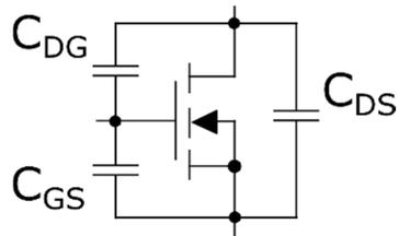
**Figure 2.6:** Capacitances for a Power MOSFET
