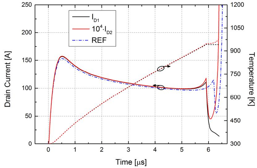
**Figure 3.13:** Simulated drain current and surface temperature
