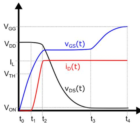
Figure 2.9: Turn-on waveforms for a power MOSFET
