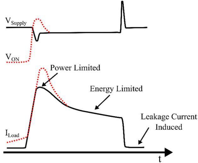
**Figure 4.1:** Typical short-circuit current and voltage waveforms
