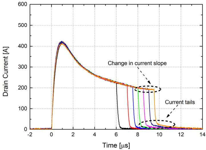
**Figure 4.6:**  $I_D$  short-circuit waveforms – SCT30N120 device
