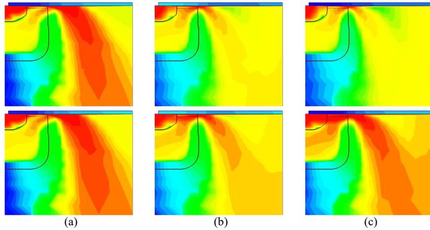
**Figure 3.14:** Current density of *cell1* (top images) and *cell2* (bottom images)
