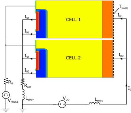
**Figure 3.12:** Diagram of mixed-mode simulated circuit.
