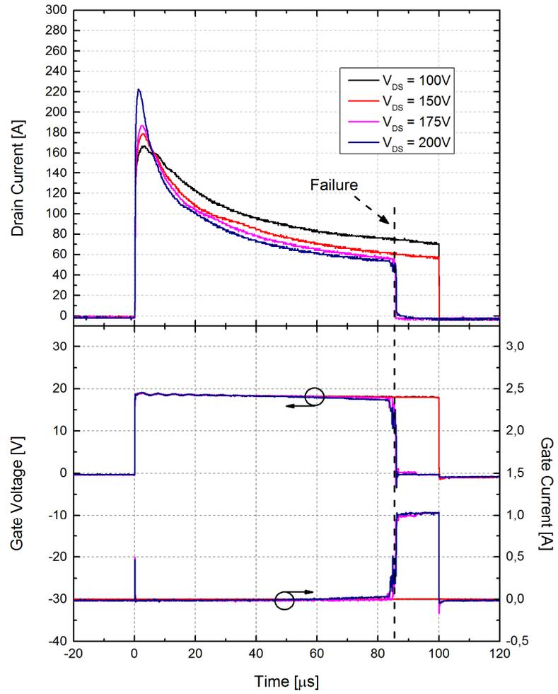
Figure 4.15:  $I_D$ ,  $V_{GS}$ ,  $I_G$  waveforms for 100 $\mu\text{s}$  pulse test
