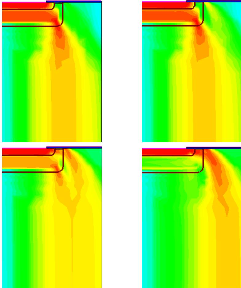
**Figure 3.22:** Current density distribution during a failed UIS test
