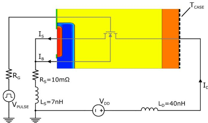
Figure 3.5: Mixed-mode simulated schematic
