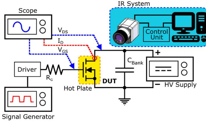
Figure 4.2: Test set-up diagram
