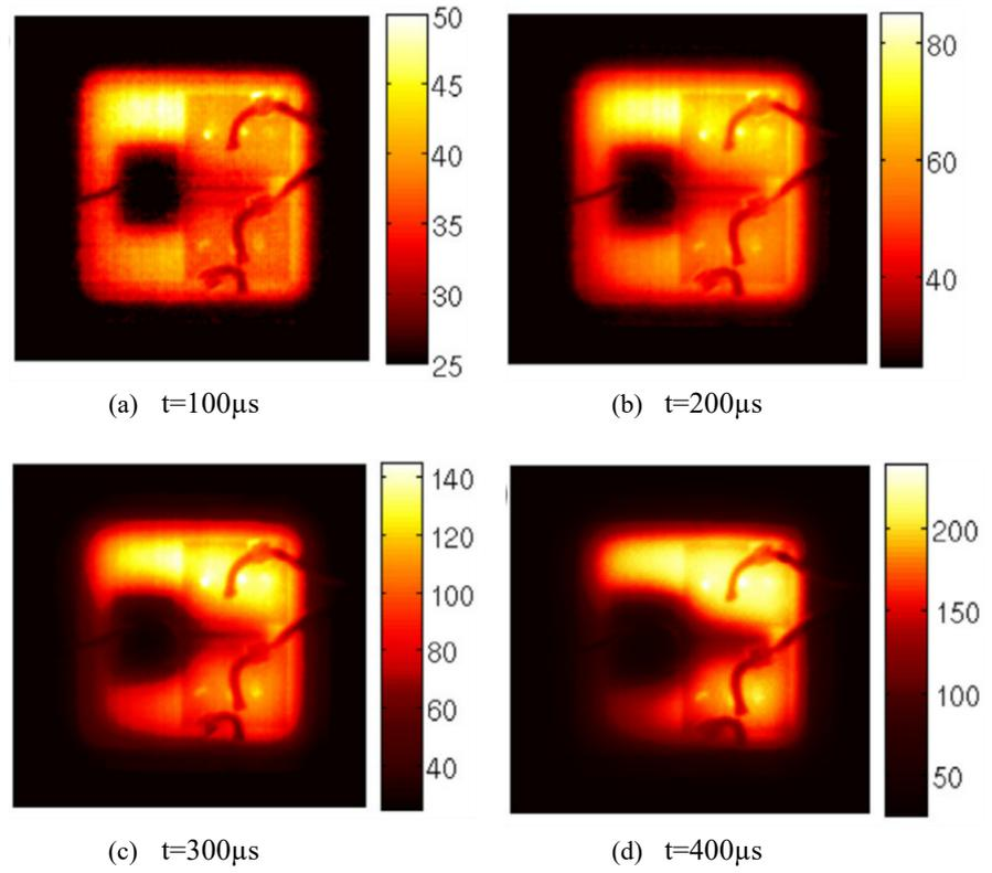
**Figure 4.19:** Temperature distribution revealing unstable operation (scale in °C)
