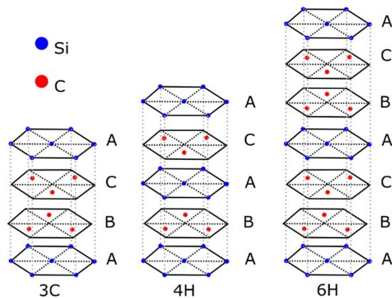
Figure 1.2: Stacking sequence for 3C-SiC, 4H-SiC and 6H-SiC
