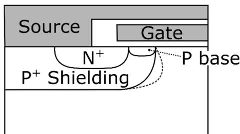
**Figure 2.2:** Detail of the shielding MOSFET structure
