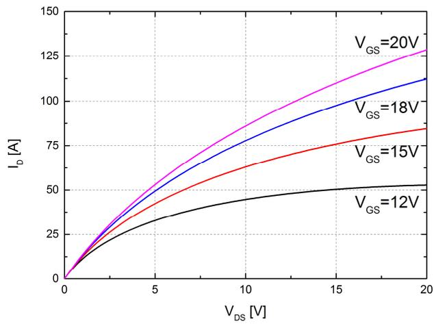
**Figure 2.4:** Typical  $I_D$ - $V_{DS}$  curves for a Power MOSFET at different  $V_{GS}$
