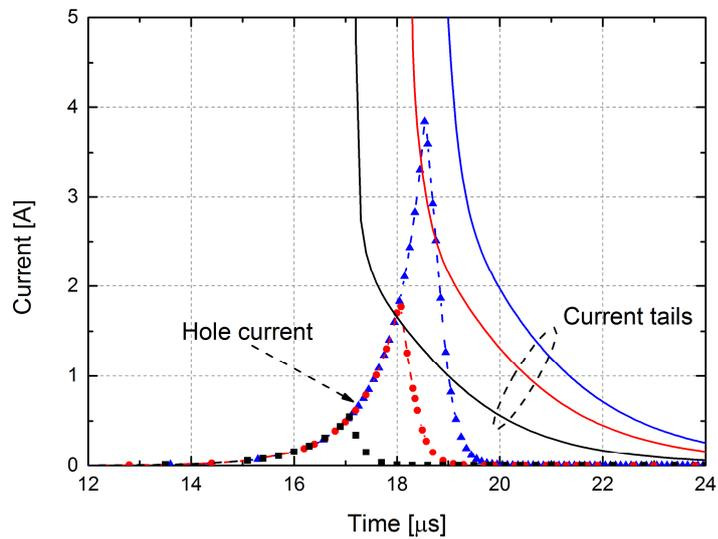
**Figure 3.7:** Detail of current tails (solid) and hole current (dashed)
