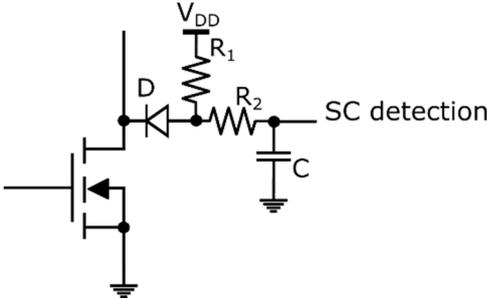
Figure C.1: Basic diagram of de-saturation technique
