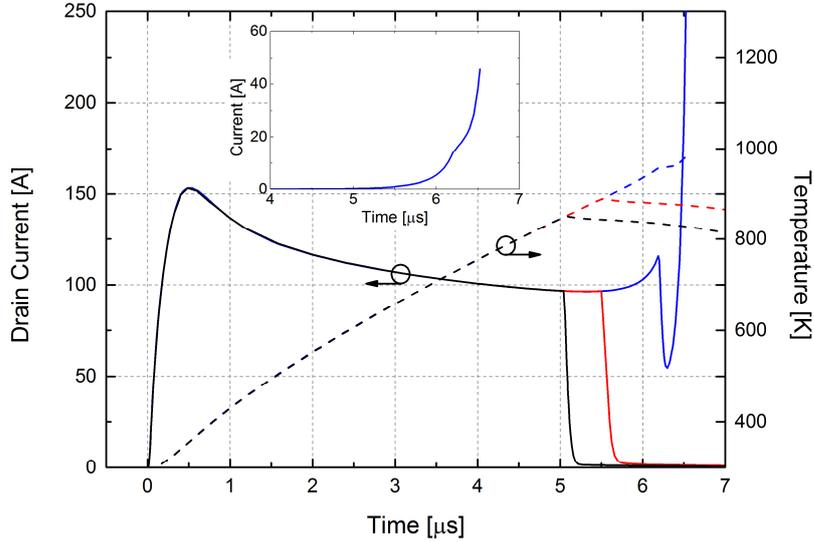
**Figure 3.11:** Simulated drain current and surface temperature. The inset shows the body terminal hole current for  $T_{\text{PUSLE}}=18.5\mu\text{s}$  ( $V_{\text{DS}}=800\text{V}$ ;  $V_{\text{GS}}=18\text{V}$ ;  $T_{\text{CASE}}=27^\circ\text{C}$ )
