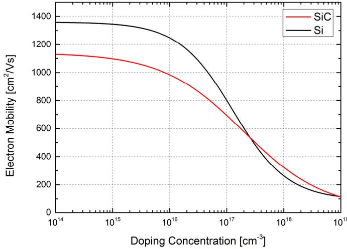
**Figure 1.5:** Electron mobility as a function of doping concentration
