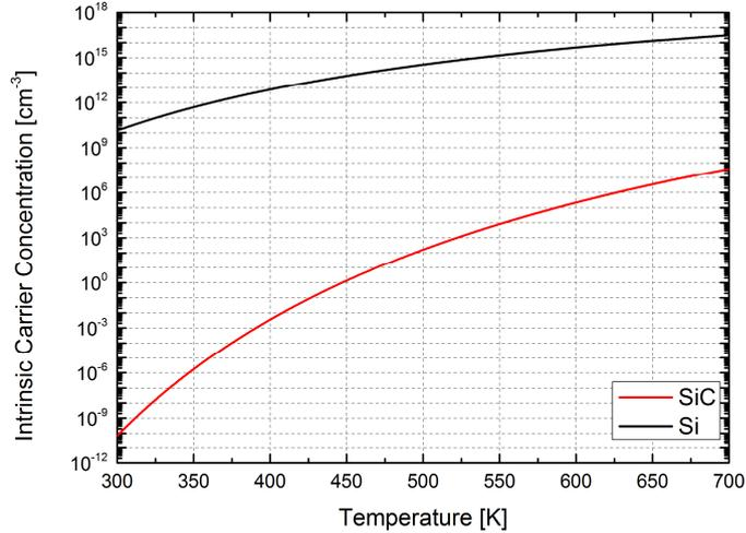
**Figure 1.3:** Intrinsic carrier concentration as a function of temperature
