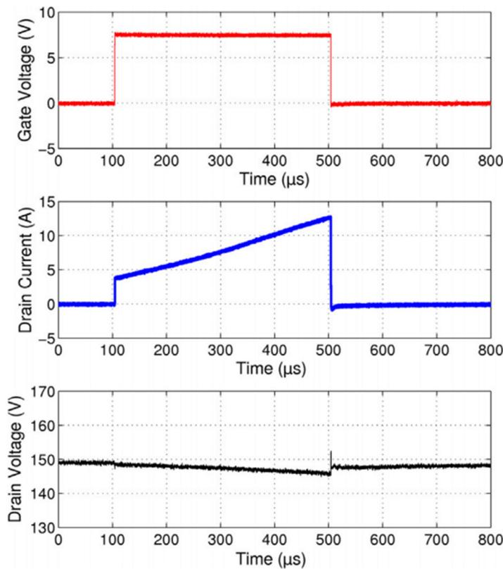
**Figure 4.18:**  $V_{GS}$ ,  $I_D$ ,  $V_{DS}$  waveforms during short-circuit unstable behaviour ( $V_{GS}=7.5\text{V}$ ,  $V_{DS}=150\text{V}$ ;  $t_{PULSE}=400\mu\text{s}$ )
