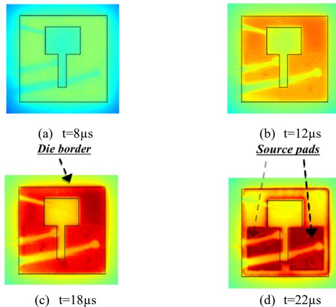
**Figure 4.14:** Normalized temperature increase
