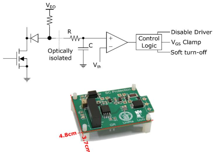
Figure C.2: Block diagram and PCB of the realized protection circuit
