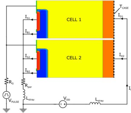
**Figure 3.12:** Diagram of mixed-mode simulated circuit. Total device is modelled with two independent parallel cells
