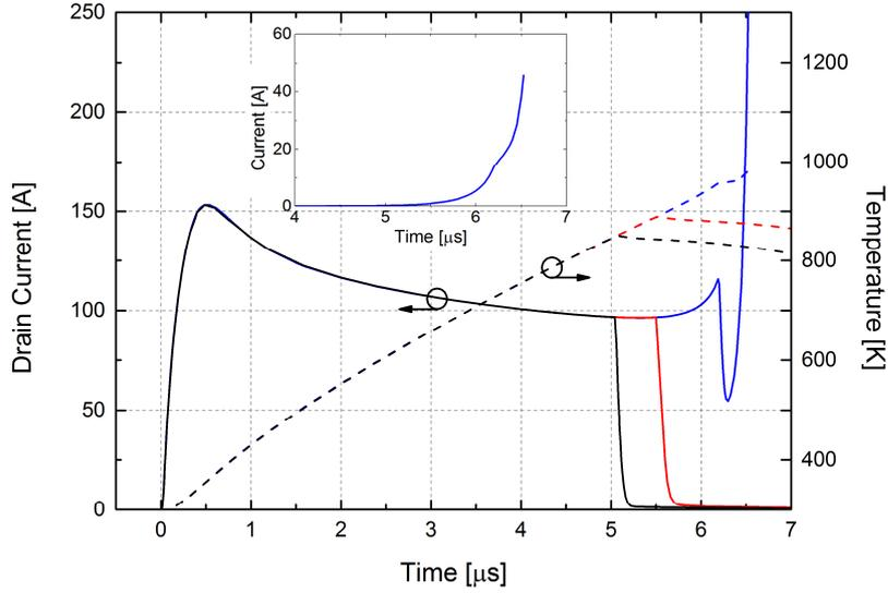
**Figure 3.11:** Simulated drain current and surface temperature. The inset shows the body terminal hole current for  $T_{\text{PULSE}}=18.5\mu\text{s}$  ( $V_{\text{DS}}=800\text{V}$ ;  $V_{\text{GS}}=18\text{V}$ ;  $T_{\text{CASE}}=27^\circ\text{C}$ )
