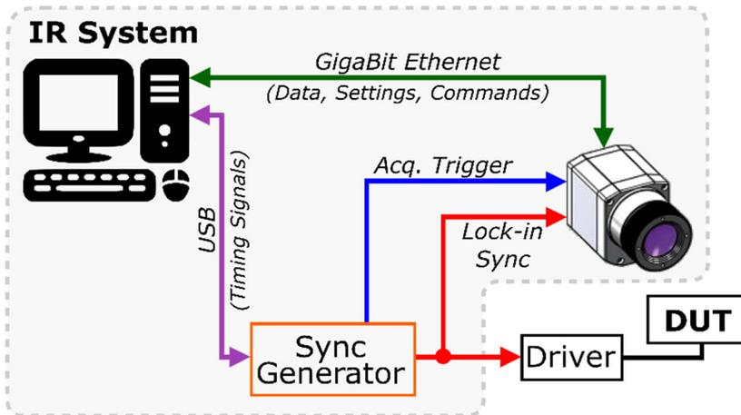
Figure A.2: Diagram of the experimental IR system
