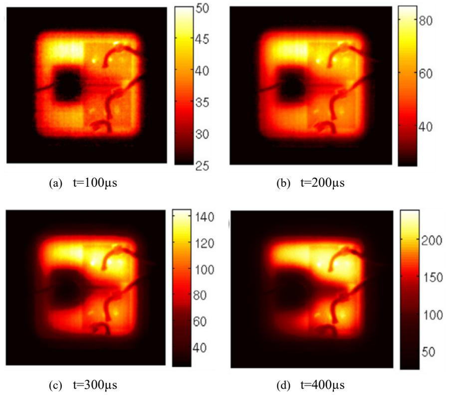
**Figure 4.19:** Temperature distribution revealing unstable operation (scale in  $^{\circ}\text{C}$ )
