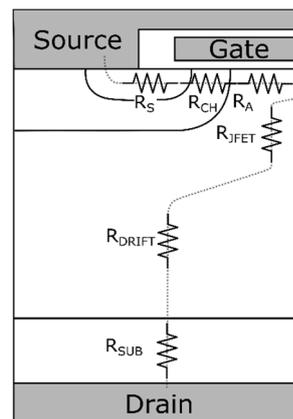
**Figure 2.3:** Different components of power MOSFET internal resistance
