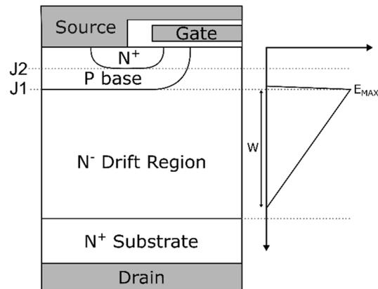
**Figure 2.12:** Schematic representation of electric field in blocking mode
