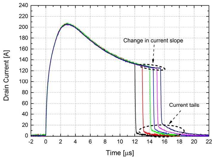
**Figure 4.7:**  $I_D$  short-circuit waveforms – SCT2080KE device
