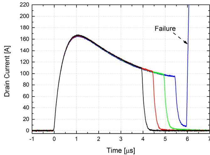
**Figure 4.11:**  $I_D$  short-circuit waveforms – C2M0080120D device
