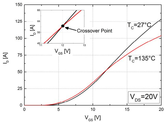
**Figure 2.5:** Typical  $I_D$ - $V_{GS}$  curves for a Power MOSFET at different temperatures
