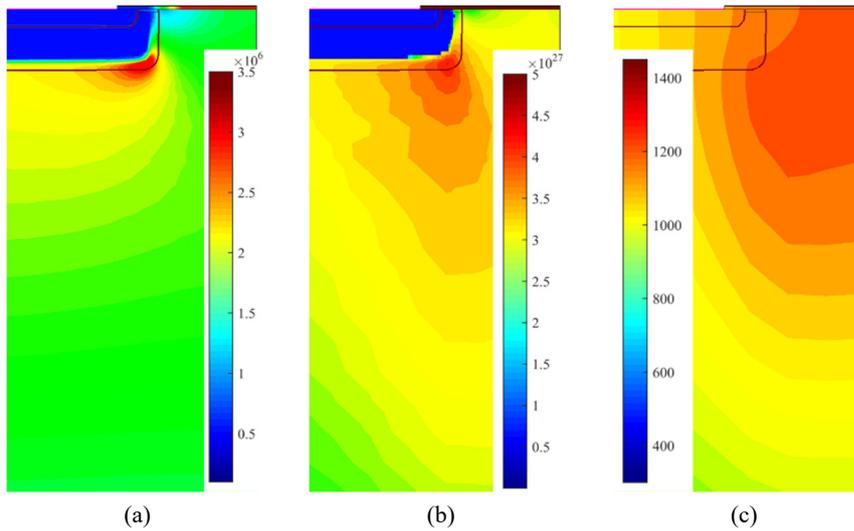
**Figure 3.21:** Distribution of electric field (a), impact ionization (b) and temperature (c)
