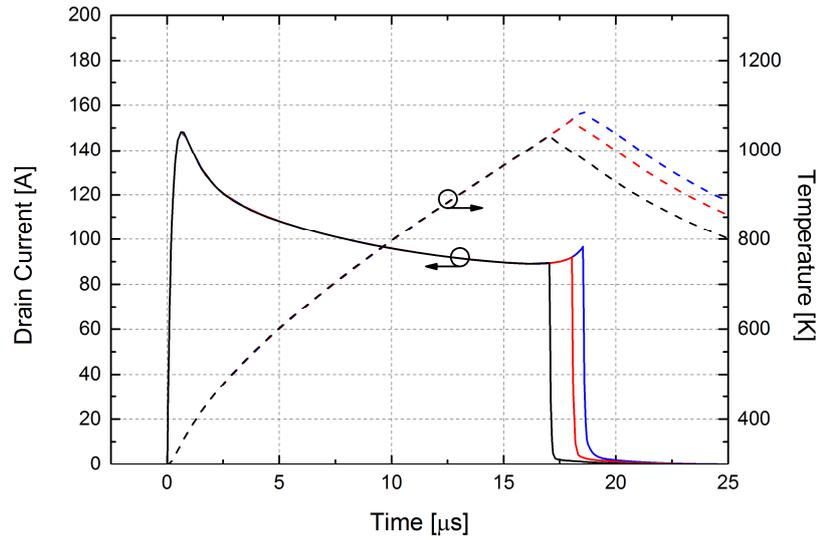
**Figure 3.6:** Simulated drain current and surface temperature ( $V_{DS}=400V$ ;  $V_{GS}=18V$ ;  $T_{CASE}=27^{\circ}C$ )
