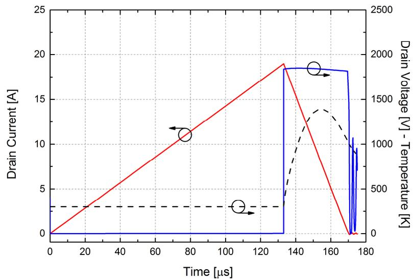
**Figure 3.20:** Simulated UIS  $I_D$  and  $V_D$  waveforms (solid) and  $T_{MAX}$  (dashed) ( $L=2.8\text{mH}$ ;  $I_{MAX}\sim 19\text{A}$ )
