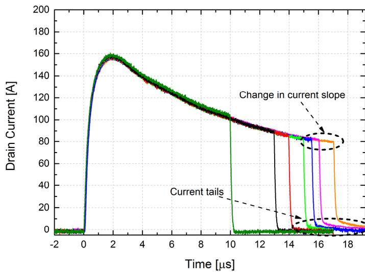
**Figure 4.3:**  $I_D$  short-circuit waveforms – C2M0080120D device
