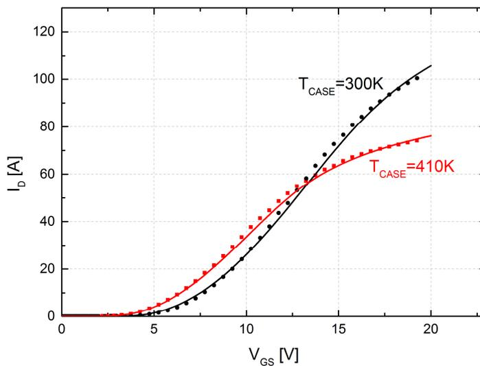
**Figure 3.4:** Measured (symbols) and simulated (solid) isothermal  $I_D$ - $V_{GS}$  characteristics ( $V_{DS}=20V$ )
