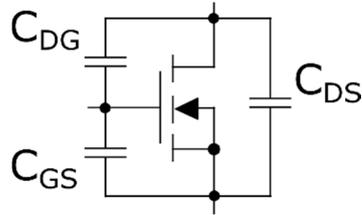
**Figure 2.6:** Capacitances for a Power MOSFET
