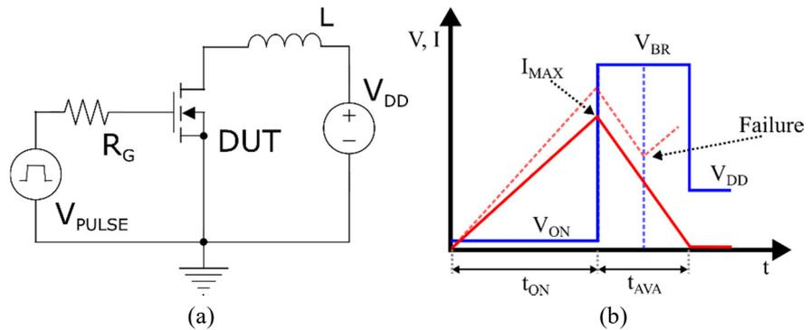
**Figure 3.19:** UIS test circuit (a) and schematic electrical waveforms (b)
