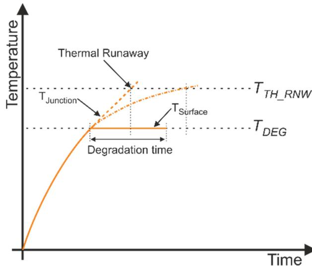
**Figure 5.2:** Failure for general applied power.
