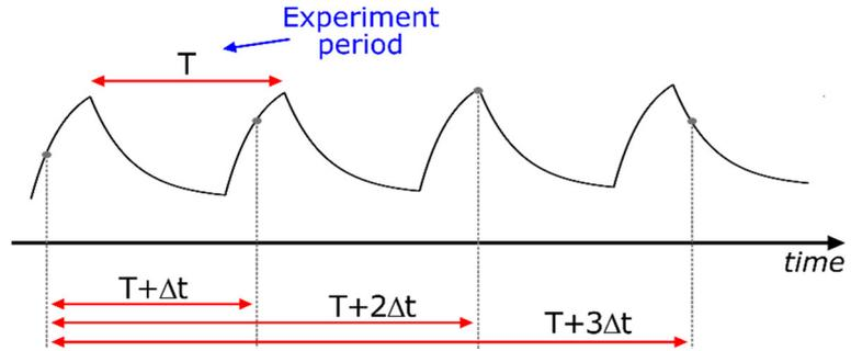
**Figure A.1:** Representation of the equivalent time sampling technique
