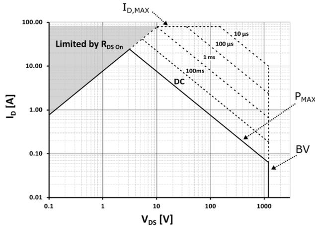
Figure 2.11: Safe Operating Area of a Power MOSFET
