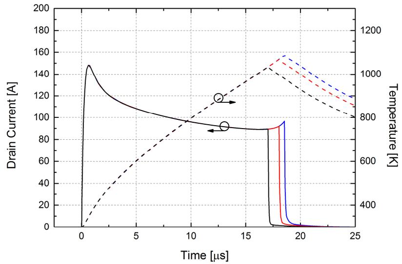
**Figure 3.6:** Simulated drain current and surface temperature ( $V_{DS}=400V$ ;  $V_{GS}=18V$ ;  $T_{CASE}=27^{\circ}C$ )
