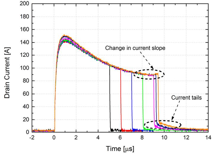
**Figure 4.4:**  $I_D$  short-circuit waveforms – C2M0080120D device ( $V_{DS}=600V$ ;  $V_{GS}=16V$ ;  $T_{CASE}=75^\circ C$ )
