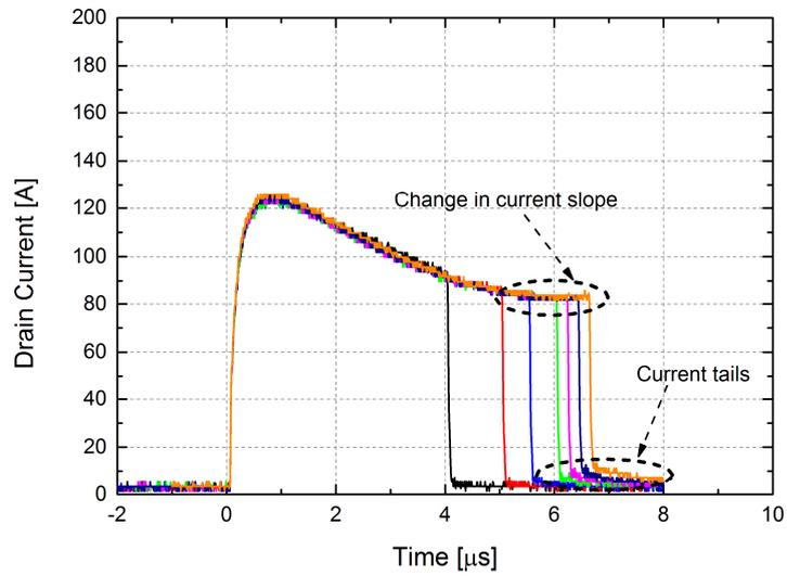
**Figure 4.5:**  $I_D$  short-circuit waveforms – C2M0080120D device ( $V_{DS}=800V$ ;  $V_{GS}=18V$ ;  $T_{CASE}=150^\circ C$ )
