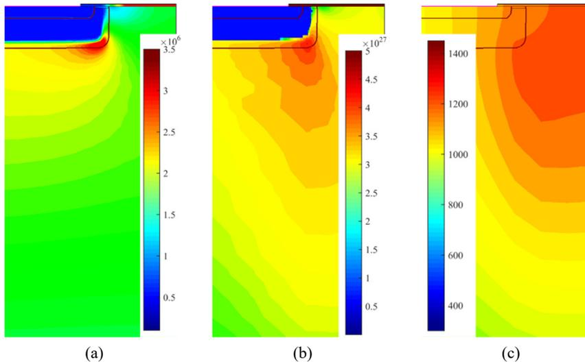
**Figure 3.21:** Distribution of electric field (a), impact ionization (b) and temperature (c)
