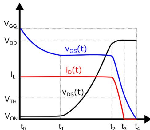
**Figure 2.10:** Turn-off waveforms for a power MOSFET
