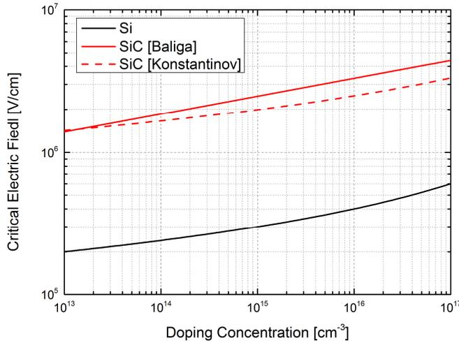
**Figure 1.4:** Critical electric field as a function of doping concentration
