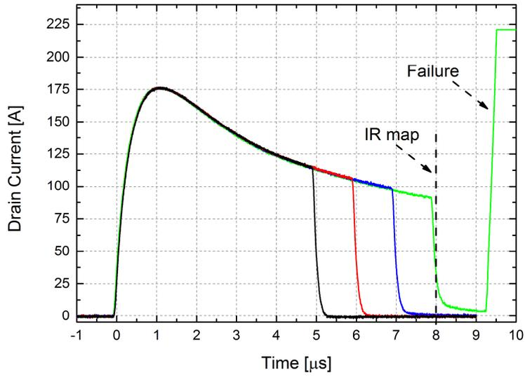
**Figure 4.9:**  $I_D$  short-circuit waveforms – C2M0080120D device
