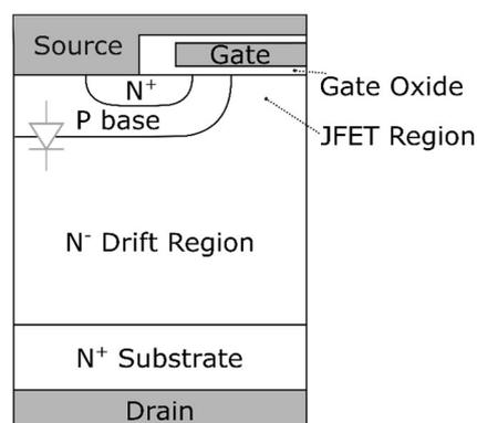
Figure 2.1: Planar MOSFET half-cell cross section
