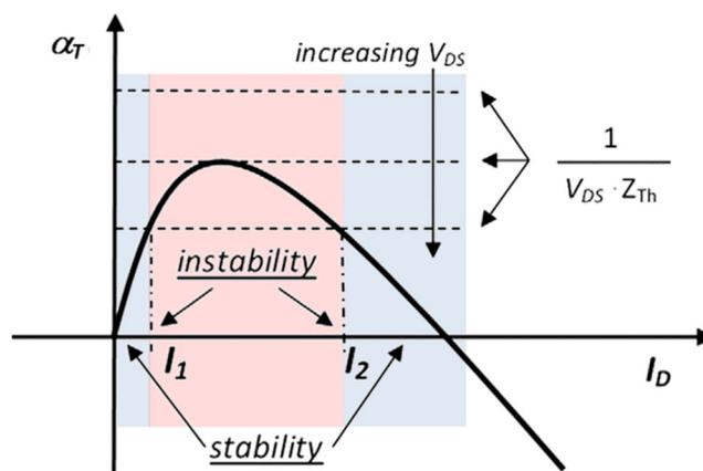
Figure 4.17: Stability graph for a power MOSFET
