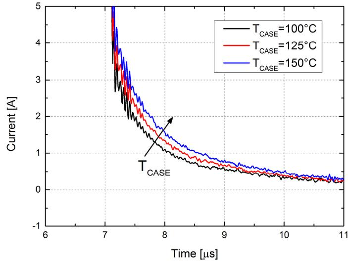
**Figure 4.8:** Current tails as a function of  $T_{CASE}$  – C2M0080120D device ( $V_{DS}=600V$ ;  $V_{GS}=18V$ )
