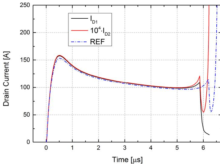
**Figure 3.15:** Simulated drain current – channel length mismatch
