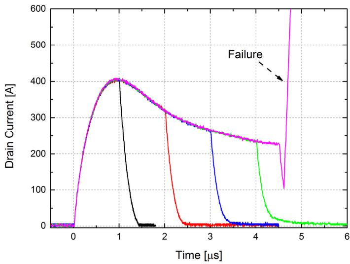
**Figure 4.10:**  $I_D$  short-circuit waveforms – SCT30N120 device
