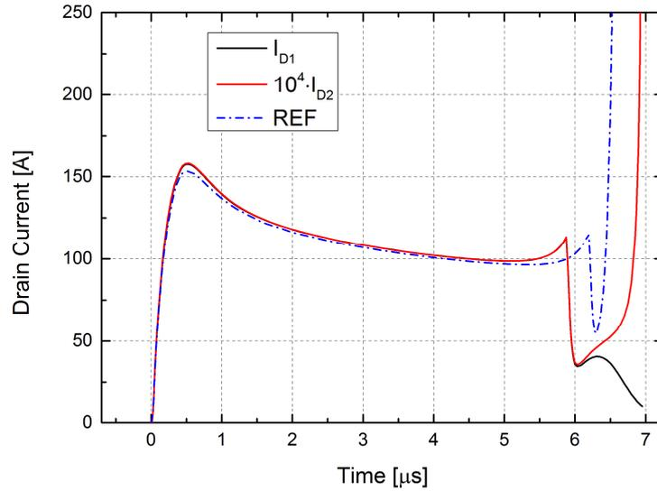
**Figure 3.16:** Simulated drain current – interface traps mismatch
