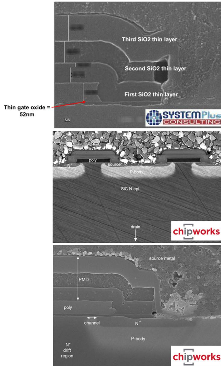
Figure 3.2: SEM cross sections used to evaluate device geometry
