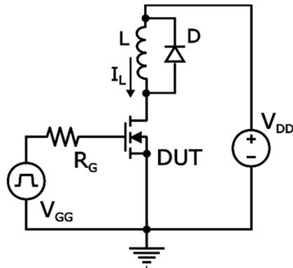
**Figure 2.8:** Simplified circuit for power MOSFET switching analysis
