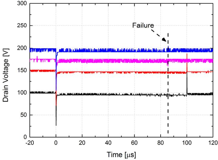
Figure 4.16:  $V_{DS}$  waveforms for 100 $\mu$ s pulse test
