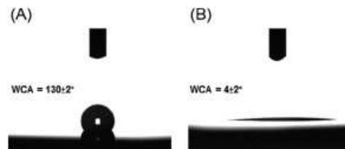
FIG. 3. Water contact angle measurements before (A) and after (B) thermal oxidation of PSi structure.
