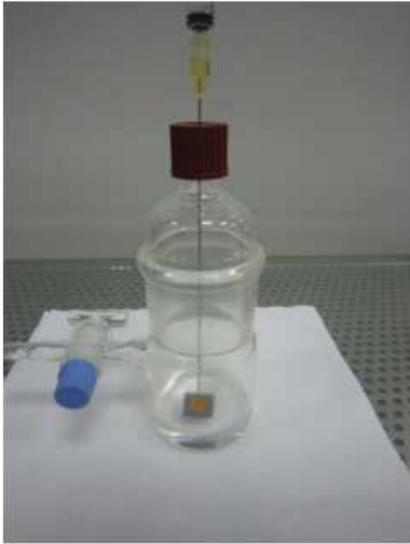
FIG. 2. Deposition chamber used for in vacuum HFBs infiltration into PSi photonic structures.
