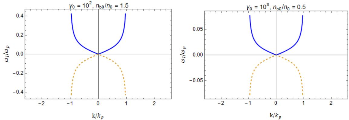
Figure 5.2: Variations of  $\bar{\omega}_I$  with  $\bar{k}$  for a monochromatic beam profile at fixed ratio  $n_{b0}/n_0$ . Here the solid lines indicate positive  $\bar{\omega}_I$  and the dashed lines indicate negative  $\bar{\omega}_I$  according to Eq. (5.3.5).
