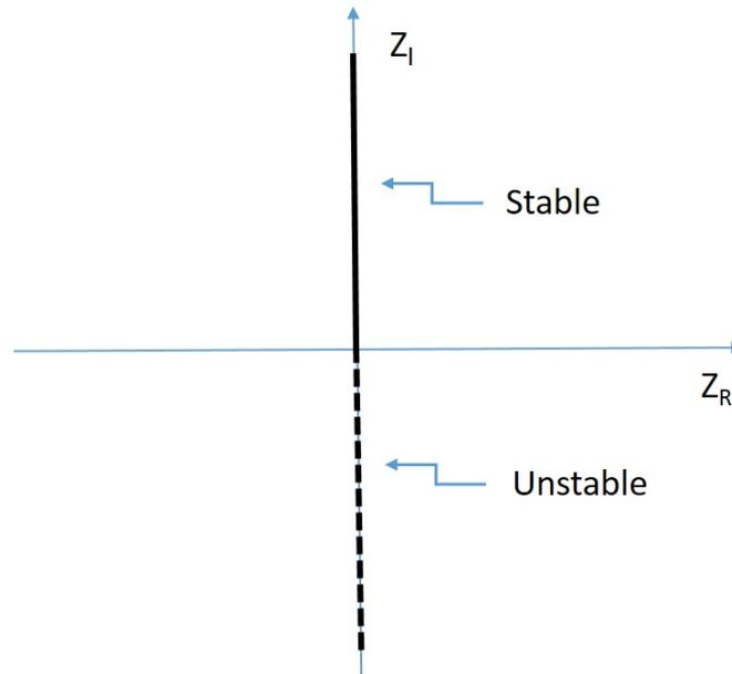
Figure 6.1: Stability analysis in the plane of the impedance for a monochromatic beam.
