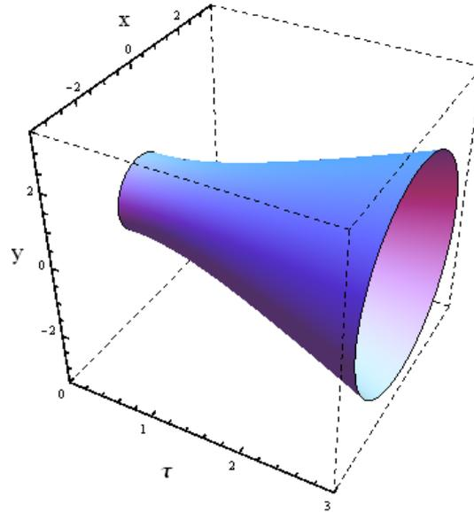
Figure 4.1: Beam envelope surface that, at each  $\tau$ , is described by  $x^2 + y^2 = \sigma_{\perp}^2(\tau)$ , for  $\mathcal{A} > 0$  (self-defocusing of the beam for  $B_0 = 0$ ). Here,  $\sigma_0 = 1$ ,  $\sigma'_0 = 0$ ,  $\tau_0 = 0$  and  $\mathcal{A} = 0.4$ .
