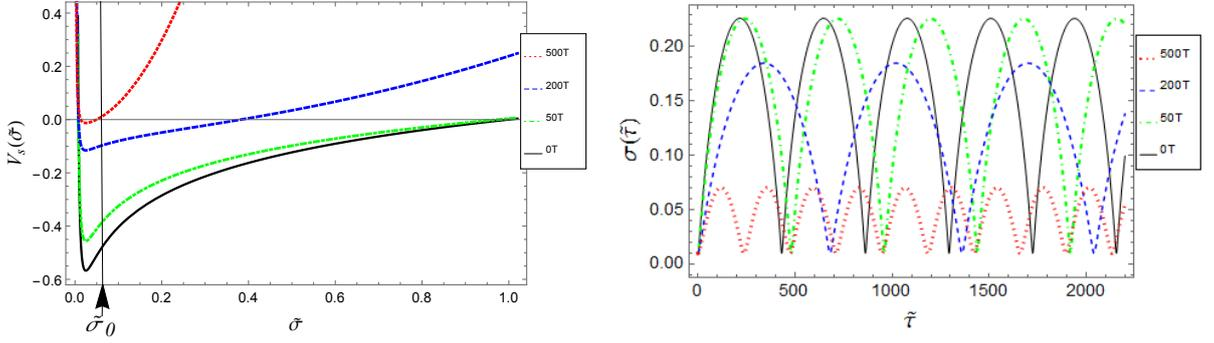
Figure 4.9: Sagdeev potential  $V_s$  as defined by Eq. (4.5.23) and corresponding oscillations of spot sizes for the different values of the external magnetic field amplitude  $B_0$ , ranging from laboratory to astrophysical environments. Initial conditions defined by  $\tilde{\sigma}_0$  sufficiently small and  $\tilde{\sigma}'_0 = 0$ . Here, the plot of  $V_s$  is scaled by a factor  $10^5$
