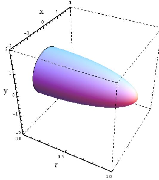
Figure 4.3: Beam envelope surface that, at each  $\tau$ , is described by  $x^2 + y^2 = \sigma_{\perp}^2(\tau)$ , for  $\mathcal{A} < 0$  (self-focusing of the beam for  $B_0 = 0$ ). Here,  $\sigma_0 = 1$ ,  $\sigma'_0 = 0$ ,  $\tau_0 = 0$  and  $\mathcal{A} = -0.5$ .
