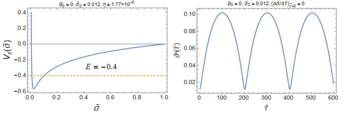
Figure 4.7: Sagdeev potential  $V_s$  (left) as defined by Eq. (4.5.23) and the corresponding numerical solution (right) of the Eq. (4.5.21) in absence of external magnetic field, where the plot of  $V_s$  is scaled by a factor  $10^5$ .
