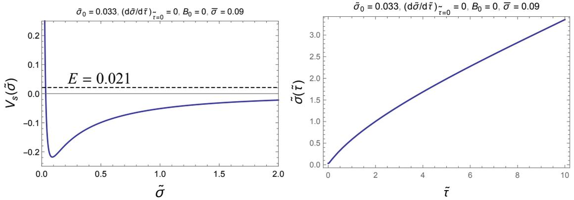
Figure 4.20: Left:  $V_s$  as function of  $\tilde{\sigma}$ , for a very small point of minimum, i.e.,  $\bar{\sigma} = 0.09$ . Right: envelope oscillations corresponding to initial conditions that fix  $E > 0$  (see left) above the plateau (i.e.,  $E = 0.021$ ), and therefore leading to an unstable evolution of the beam envelope, starting from values of  $\tilde{\sigma}_0$  sufficiently small between the asymptote around zero and  $\bar{\sigma}$ .
