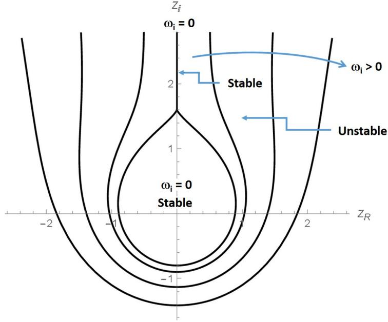
Figure 6.2: Qualitative plot of the contours in the plane  $(Z_R, Z_I)$ , generated by the mapping (6.5.7) for different constant instability growth rates  $\omega_I$ , for a thermal distribution given by (6.5.6). The stability region is surrounded by the curve  $\omega_I = 0$ .
