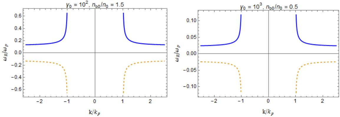
Figure 5.1: Variations of  $\bar{\omega}_R$  with  $\bar{k}$  for a monochromatic beam profile at fixed ratio  $n_{b0}/n_0$ . Here the solid lines indicate positive  $\bar{\omega}_R$  and the dashed lines indicate negative  $\bar{\omega}_R$  according to Eq. (5.3.4).
