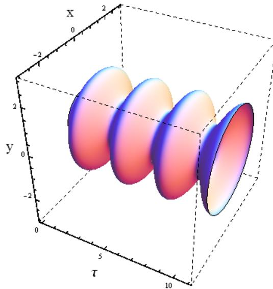
Figure 4.6: Beam envelope surface that, at each  $\tau$ , is described by  $x^2 + y^2 = \sigma_{\perp}^2(\tau)$ , for  $\mathcal{A} > K\sigma_0^2/2$  (beam self-modulation, i.e., betatron-like oscillation, for  $B_0 \neq 0$ ). Here,  $\sigma_0 = 1$ ,  $\sigma'_0 = 0$ ,  $K = 1$  and  $\mathcal{A} = 2.5$ .
