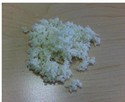
**Figure 24.** Chopped polyurethane foam with immobilized enzyme
