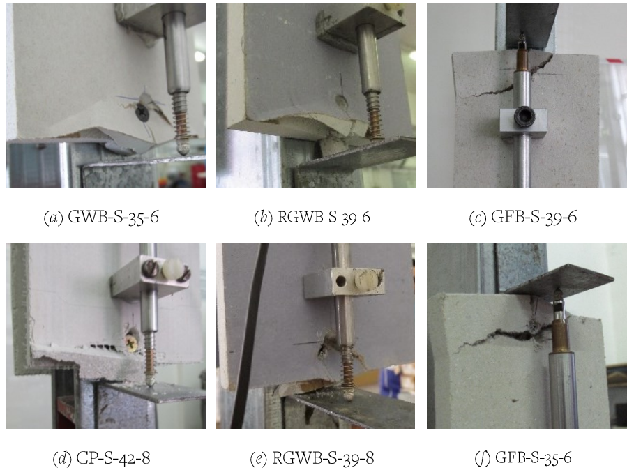
Fig. 6.9: Breaking of the sheathing edge for connections with single layer of panels
