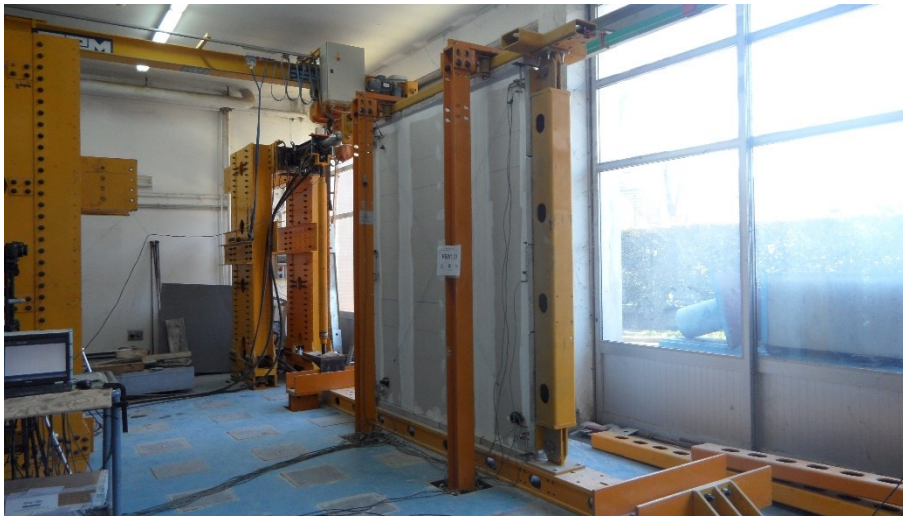
Fig. 4.6: In-plane tests on lightweight steel drywall partition walls
