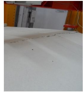
C. Panel flexural breaking
