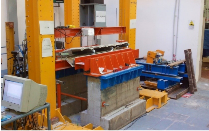
Fig. 7.21: Collapse of a tested “short partition wall”
