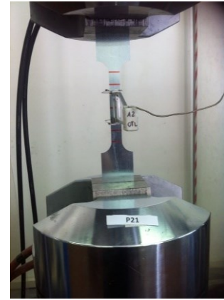
Fig. 5.2: Instrumentation for tensile tests
