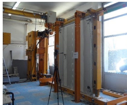
Fig. 8.2 In-plane tests on full-scale partition walls
