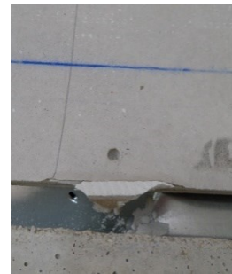
E. Failure of panel-to-frame connections
