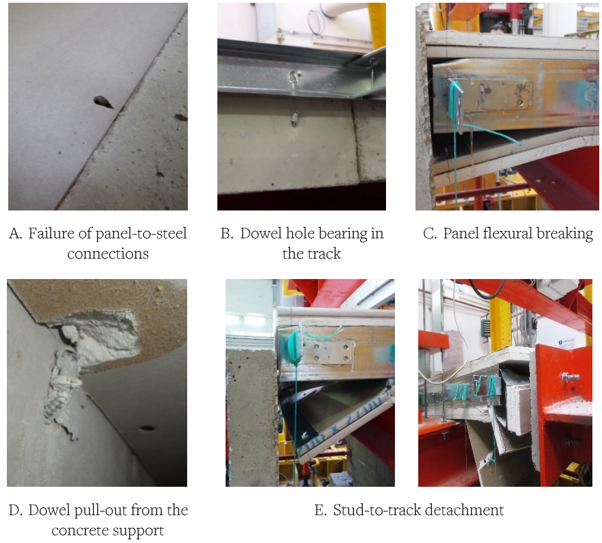
Fig. 7.19: Load vs. displacement curve and observed failure mechanisms
