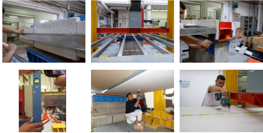
Fig. 7.6: Installation procedure of the tested partition walls
