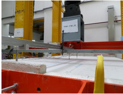
Fig. 7.13: Adopted linear variable differential transducers
