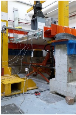
Fig. 7.12: Adopted linear wire potentiometers
