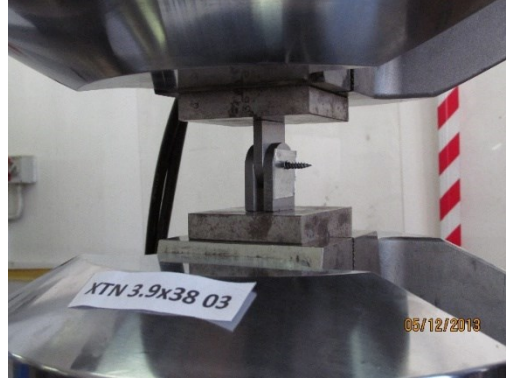
Fig. 5.9: Test set-up for shear tests on screws
