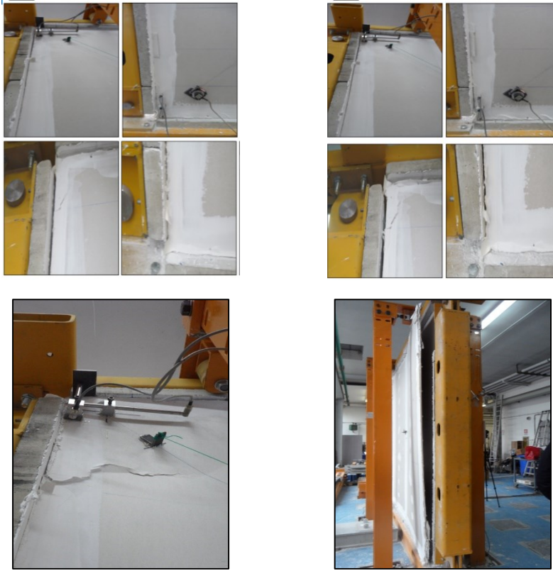
Fig. 8.9: Observed damage for test FSW1_02: a) drift level of 1.37%; b) drift level of 2.13%; c) drift level of 2.84%
