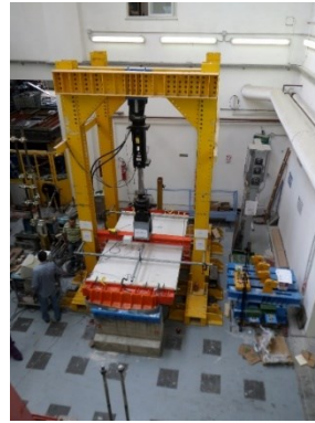
Fig. 7.2: Out-of-plane tests on full-scale partition walls
