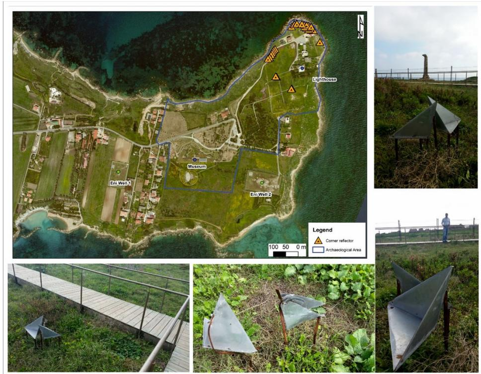
**Figure 7.14** Location of the corner reflectors installed. All around, photos of some of the corners.
