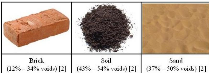
Fig. 1. Examples of porous materials.
