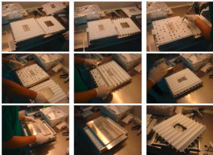
Figure 3.10: Steps of assembly. From left to right and top to bottom: half layer is arranged on the jig; teflon mask is aligned; glue spots are applied; mask is removed; bars of the other half layer are placed; second jig is applied on top to align last half layer and to distribute pressure; half module as it appears the day after gluing.
