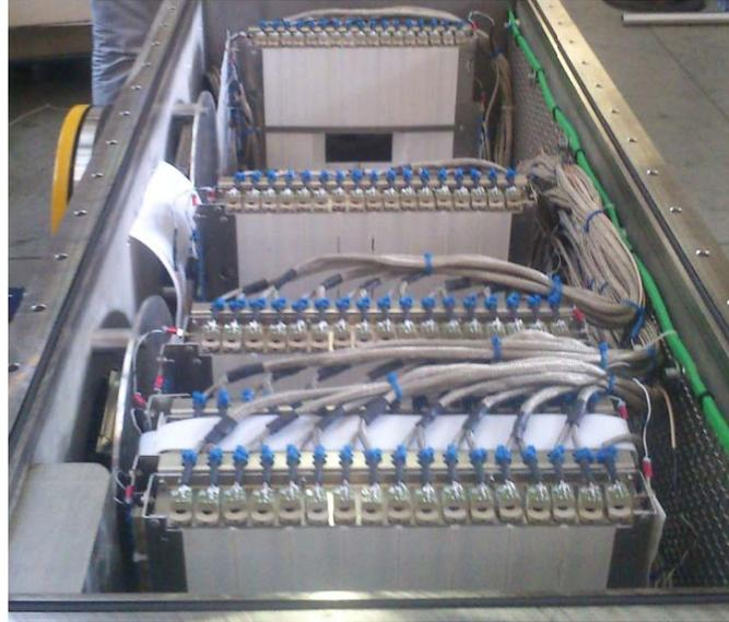
Figure 5.1: The first five CHANTI stations assembled in their vacuum vessel.
