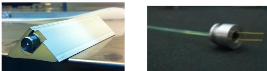
Figure 3.5: Left: bar shape. Right: Fiber connector with SiPM.
