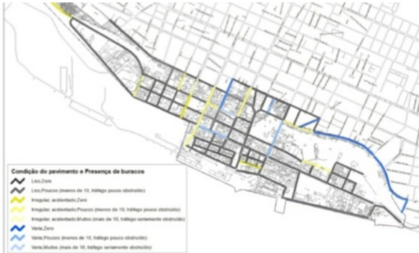
Figure 5.40 – Physical condition of roads network
