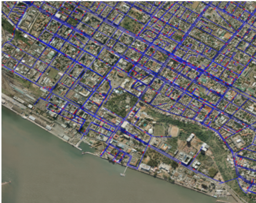
Figure 5.33 – Existing water supply infrastructure within the Baixa
