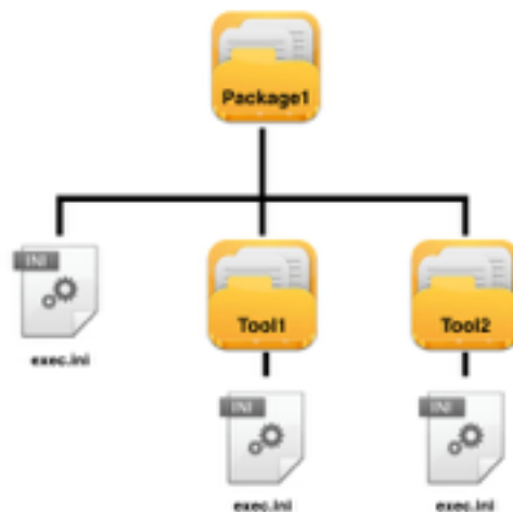
Figure 12. Hierarchy structure of configuration files for a package.
