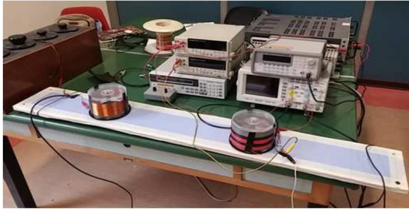
Fig 4.35. Two coils setup arrangement during test and prototyping operations.
