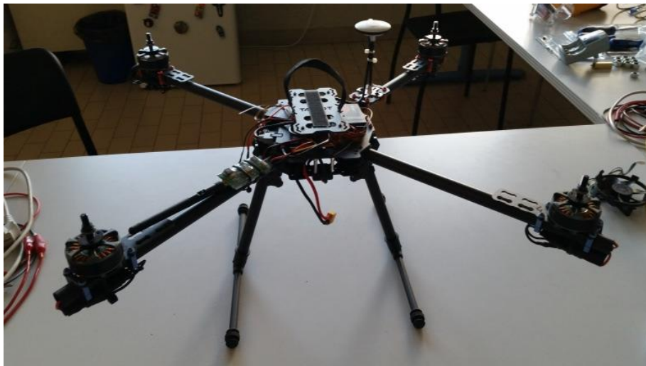
Fig. 4.21. The helicopter equipped with the prototype induction based recharge system.
