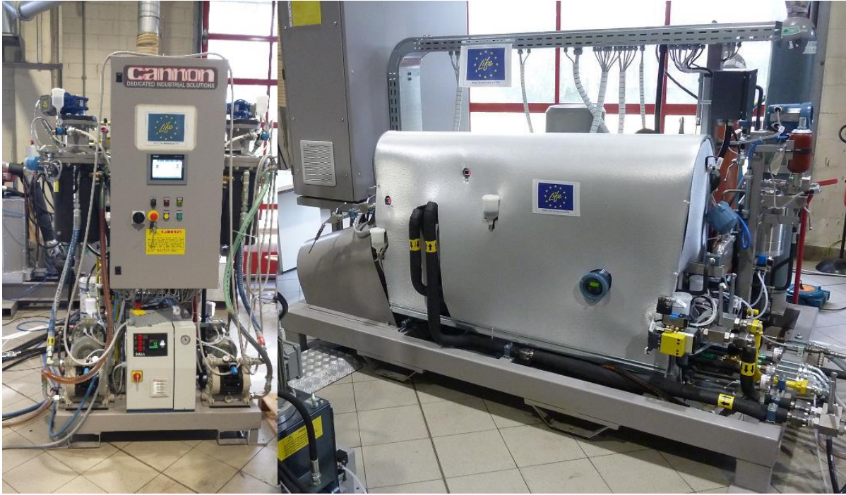
Fig. 13: Pilot plant for PUR foaming technology at Afros-Cannon facility.
