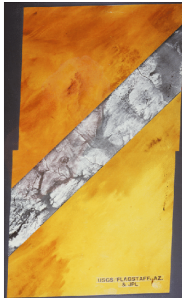
Figure 3.2. A radar scan from the shuttle in band L (SIR-A) of the African Sahara, in comparison with an optical image from Landsat ETM+ (image courtesy of JPL).
