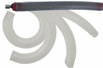
Figure 6.23: Example of soft bending actuators. Picture from the soft robotics toolkit<sup>a=</sup>
