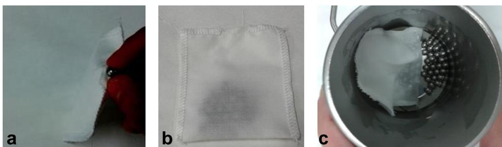
**Figure S2.6.** Preparation of fabric samples for the industrial washing process: a) insertion of stainless steel in the fabric; b) fabric bag with 25 stainless steel inside; c) view of the inside part of the apparatus used for the washing process.
