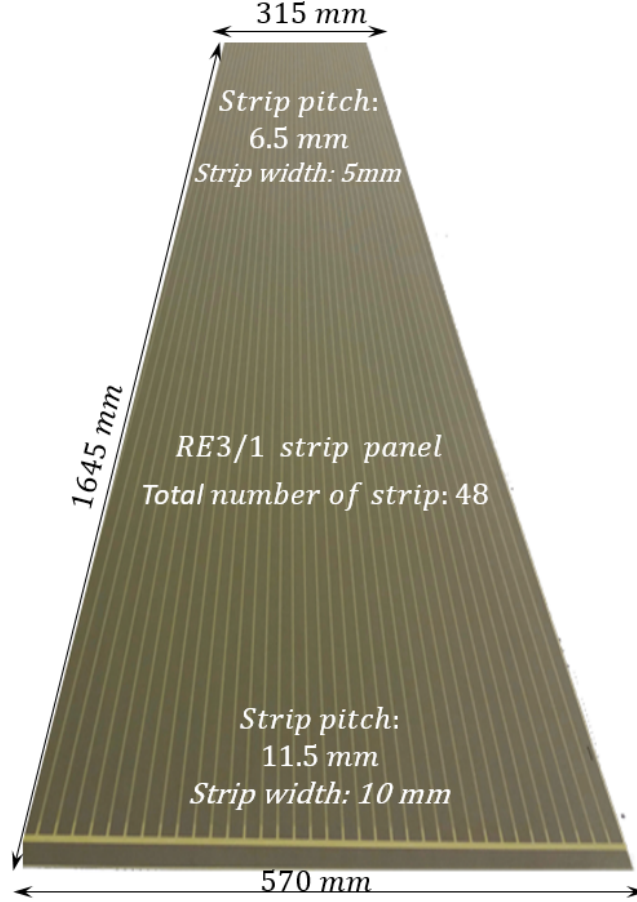
Figure 6.1: Picture of readout strip panel with its main characteristics for the iRPC RE3/1 detector prototype.
