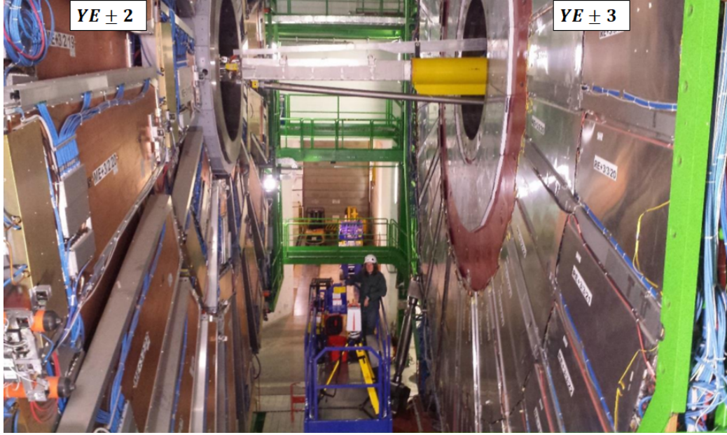
Figure 5.9: Survey campaign for the future iRPC RE+3/1 station installation in the Yoke Endcap \pm 3 iron disk.
