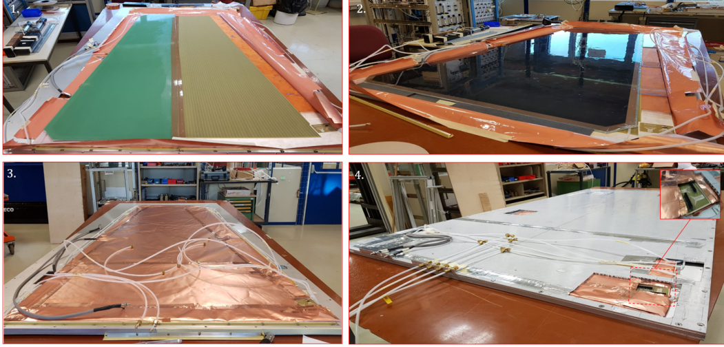
Figure 6.16: Few steps of the iRPC RPC RE4/1 detector prototype assembly procedures: 1 - installation of readout and fake strip panel; 2 placing of top gas gap and fixing it by using the polycarbonate spacers; 3 - closing the Faraday cage; 4 - the completed of the iRPC RE4/1 detector prototype assembly and flushing gas gaps.
