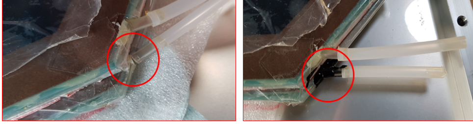
Figure 7.7: Pictures of the problematic gas nozzle of the bottom gap (a) and view of this gas nozzle after repair procedure (b).
