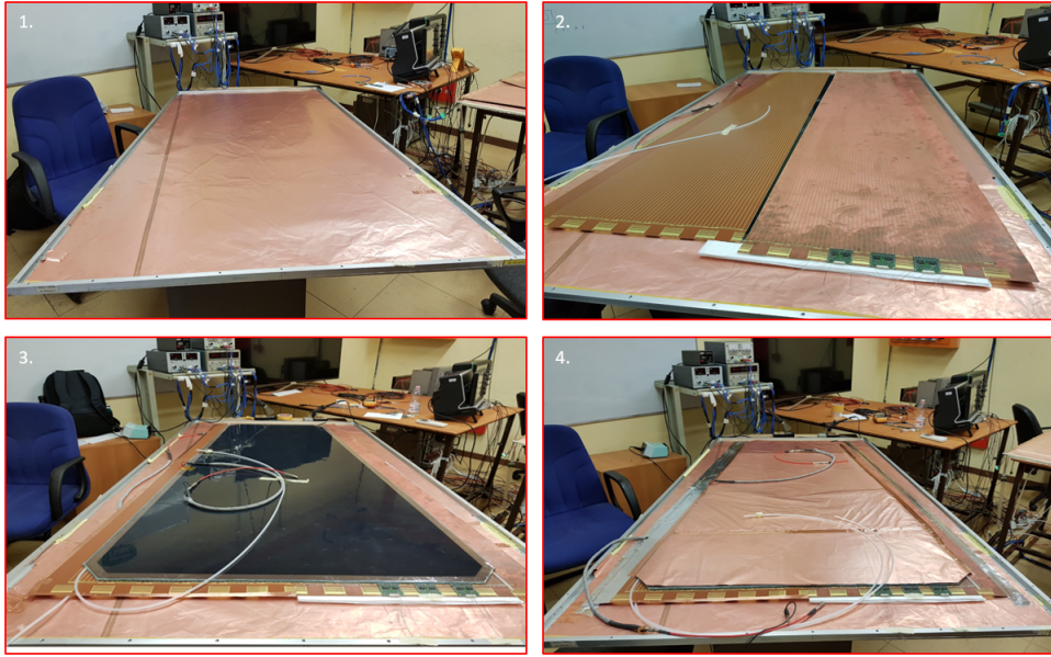
Figure 7.11: Pictures of the several assembly steps of the iRPC RE4/1 detector prototype at the INFN Rome Tor Vergata Laboratory: 1 - preparation of detector casing by covering it with a Maylar layer and the bottom copper sheet for Faraday cage; 2 - installation of bottom gas gap and readout strip panel with connected INFN Rome electronics; 3 - placing of top gas gap; 4 - closing of Faraday cage by using the copper tapes.
