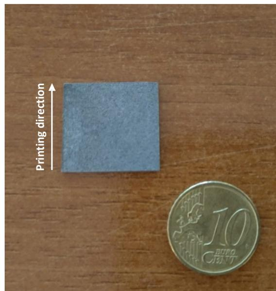
**Figure 5.1.** Illustration of an AlSi10Mg squared flat sample produced in collaboration with MBDA Italy S.p.A through SLM technology (a 10 cents coin is reported as a scale marker).
