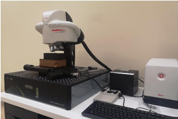
**Figure 5.3.** Leica DCM3D confocal microscope.
