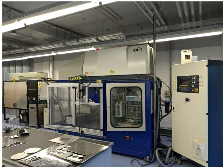
**Figure 8.1.** Rofin DC-015 CO<sub>2</sub> laser.
