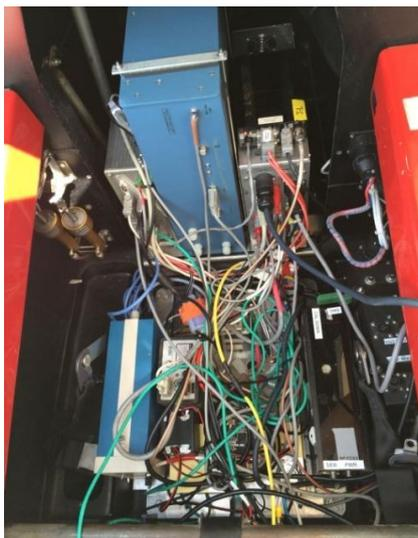
**Figure 1.2** *The air quality payload on board the Sky Arrow ERA*
