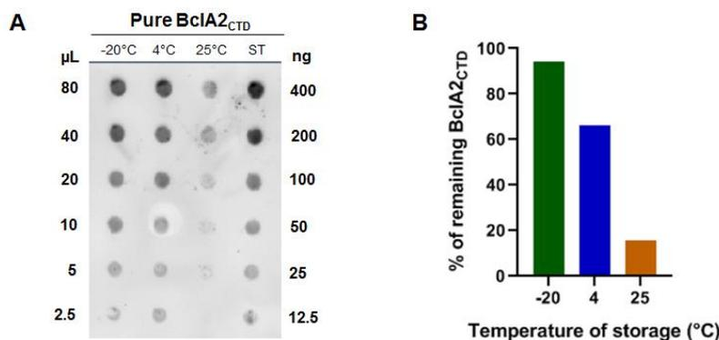
**Figure 1.2. Stability of purified BclA2<sub>CTD</sub>.** (A) Dot blotting of purified BclA2<sub>CTD</sub> stored for 2 days at -20°C, +4°C or at +25°C with anti-6xHis antibody. The protein stored at -80°C right after purification (ST) was considered as standard. Loaded volumes of purified protein (μL) and known amount of the standard (ng) are indicated. (B) Plot of the densitometric analysis of dot blot experiment of panel A, considering the amount of protein stored at -80°C as 100%.
