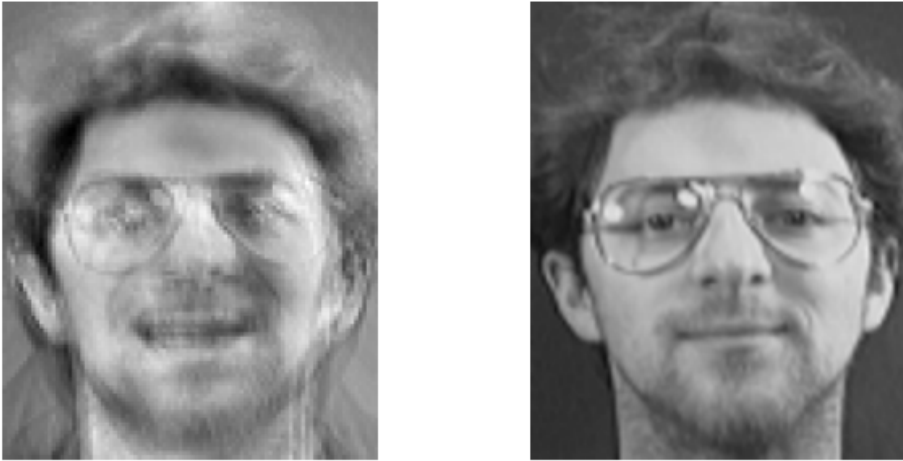
Figure 1.11: Illustrative example of a model inversion attack against a CNN-based face authorisation system: on the left, the sample reconstructed by the attack; on the right the actual subject sample. To perform the attack, the attacker only needs the target subject id and the ability to query the authorisation system to obtain the confidence score (image from [53]).
