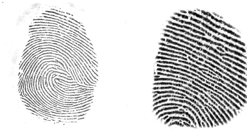
Figure 5.10: Example of different geometric distortions introduced by acquiring the same fingerprint by using two different scanners: GreenBit (left) and DigitalPersona (right).
