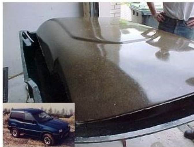
Fig.14: Application of natural fibres as roof in automotive field.
