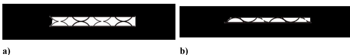
Fig.27: Core configurations: peak to peak assembly (a); peak to valley assembly (b).
