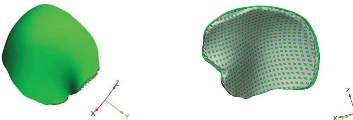
**Figure 2.5.** 3D geometrical models of a customized hybrid device for large cranial defect: top view evidencing the external cement layer (left); bottom view highlighting the cement infiltration in the fully interconnected pore network. Green color was chosen to identify the cement component of the hybrid device.
