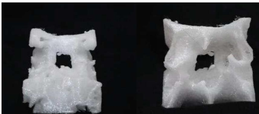
**Figure 3.9.** 3D Additive manufactured model of a skull base region with the created defect – different views.
