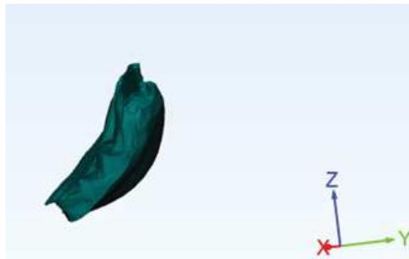
**Figure 3.7.** 3D model of the customized device as closure system for the skull base defect.
