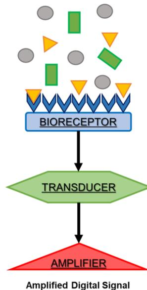
**Figure [1.2] Schematic representation of a biosensor.**
