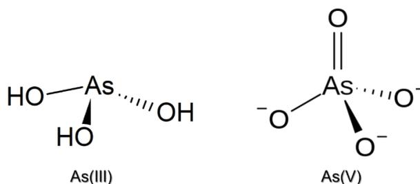
Figure [1.1] Structures of the most common forms of inorganic arsenic: As(III) and As(V).
