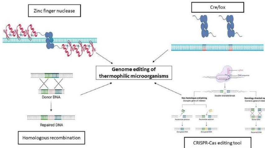
**Figure 5.** Schematic representation of the genome editing tools for thermophilic microorganisms. The Zinc finger nuclease is the first genome editing tool setup for thermophilic microorganisms. The most common is the spontaneous homologous recombination. In the last decades, the Cre/lox and CRISPR-Cas based tools were adapted for thermophiles (Created with BioRender.com (accessed on 20 January 2021)).
