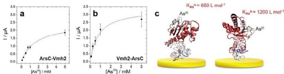
**Figure 6.** Evolution of the SWV peak current towards starting As(III) concentrations. (a) ArsC-Vmh2-modified gold electrode and (b) Vmh2-ArsC-modified gold electrodes accompanied by a schematic representation of arsenic binding (c). The red line corresponds to the curve fitting using Eq. (2).
