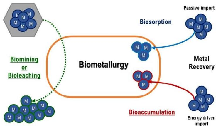
**Figure 2.** Schematic representation of metal bioprocesses in biometallurgy. Metals (blue circles) can be extracted from ores through biomining/bioleaching (green arrow) and they can be recovered into the cell by passive import (biosorption—blue arrow) or energy driven transport (bioaccumulation—red arrow).
