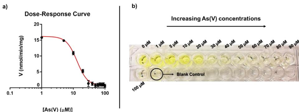
**Figure 6. a)** Dose-response curve of the inhibition of *TtArsC* phosphatase activity at increasing concentration of As(V), reported in panel b). **b)** *TtArsC* phosphatase activity assay in multiwell plate at increasing concentrations of As(V).
