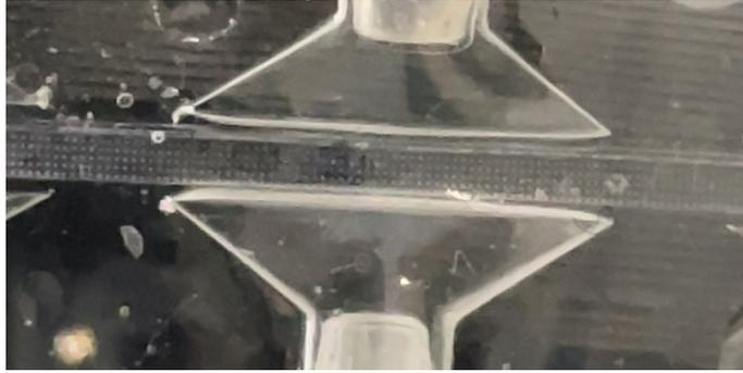
*Figure 73. Schematic representation of ‘Peristalsis on a chip’ with integrated PDMS membrane.*
