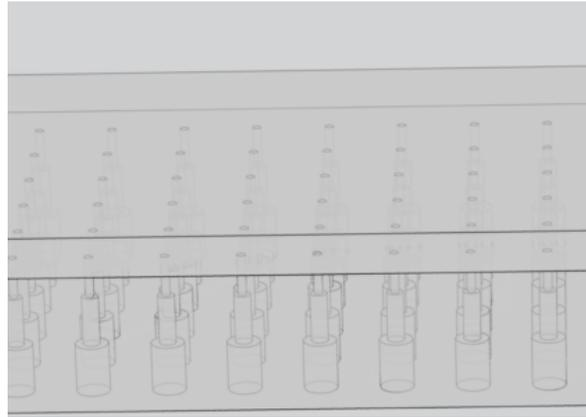
Figure 29. Scheme of PDMS Conventional membrane, 20 $\mu\text{m}$  pores exposed, integrated in microchannel.
