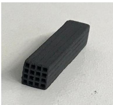
**Figure 2. 1.** Monolith obtained by cutting the original sample provided by Helsa Functional Coating
