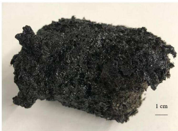
**Figure 3. 5** Foamy PFA obtained from Zn-activated polymerization of FA at 80 °C
