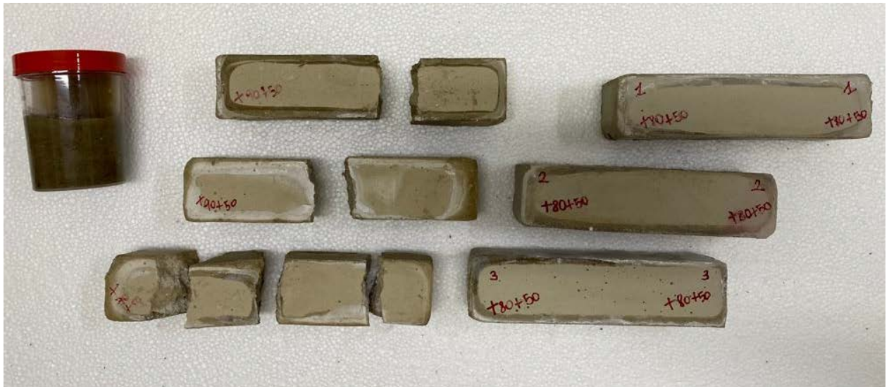
Figure n. 51 - Prismatic tuff samples
