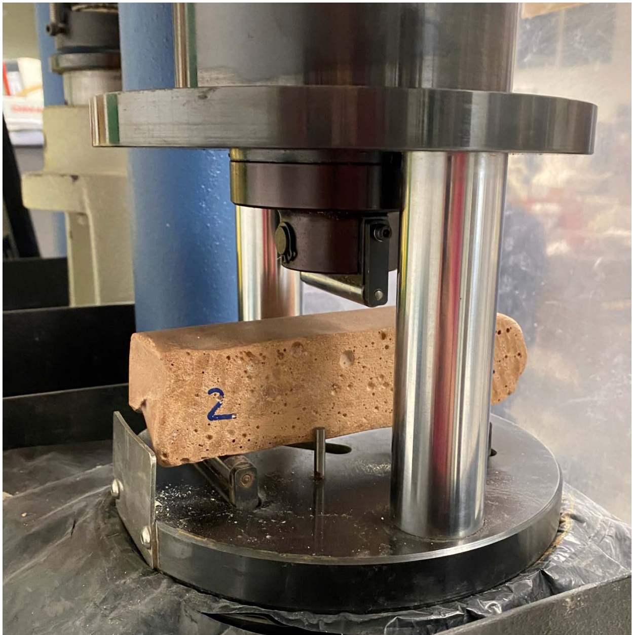
Figure n.31 - Performing flexural strength tests on geopolymer samples
