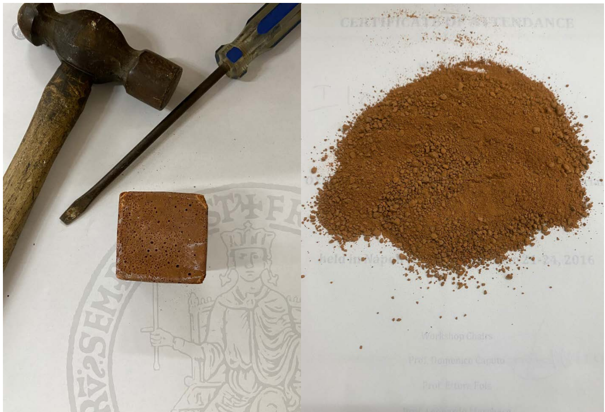
Figure n.117 - Crushing of sample CP 80% for re-geopolymerisation test
