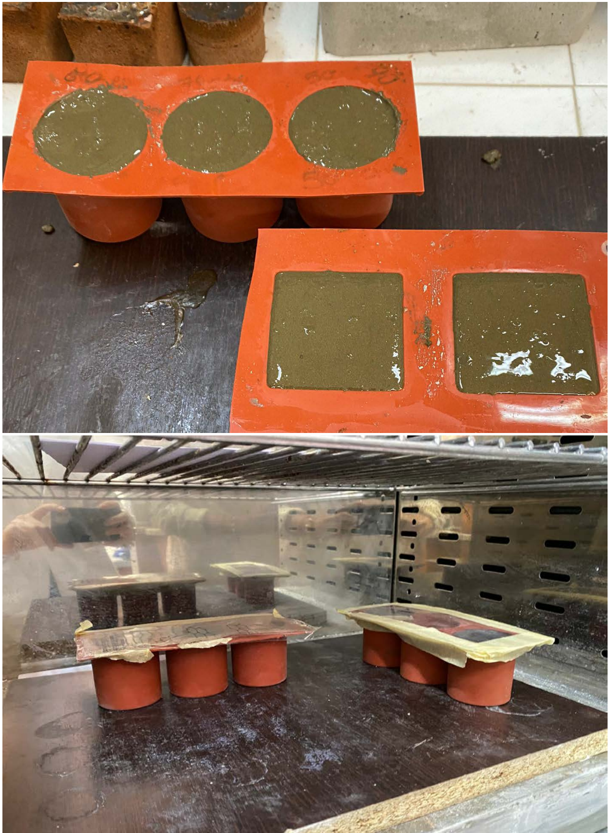
Figure n.27 - Mixtures poured into the cubic and cylindrical moulds for the production of physical test specimens and subsequently baked
