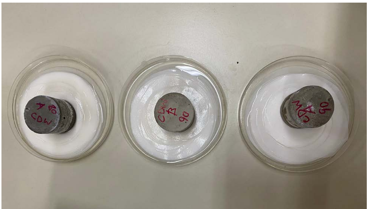
Figure n.102 - Samples subjected to capillary absorption test
