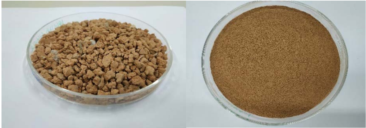
Figure n.152 - Waste before (a) and after grinding (b)
