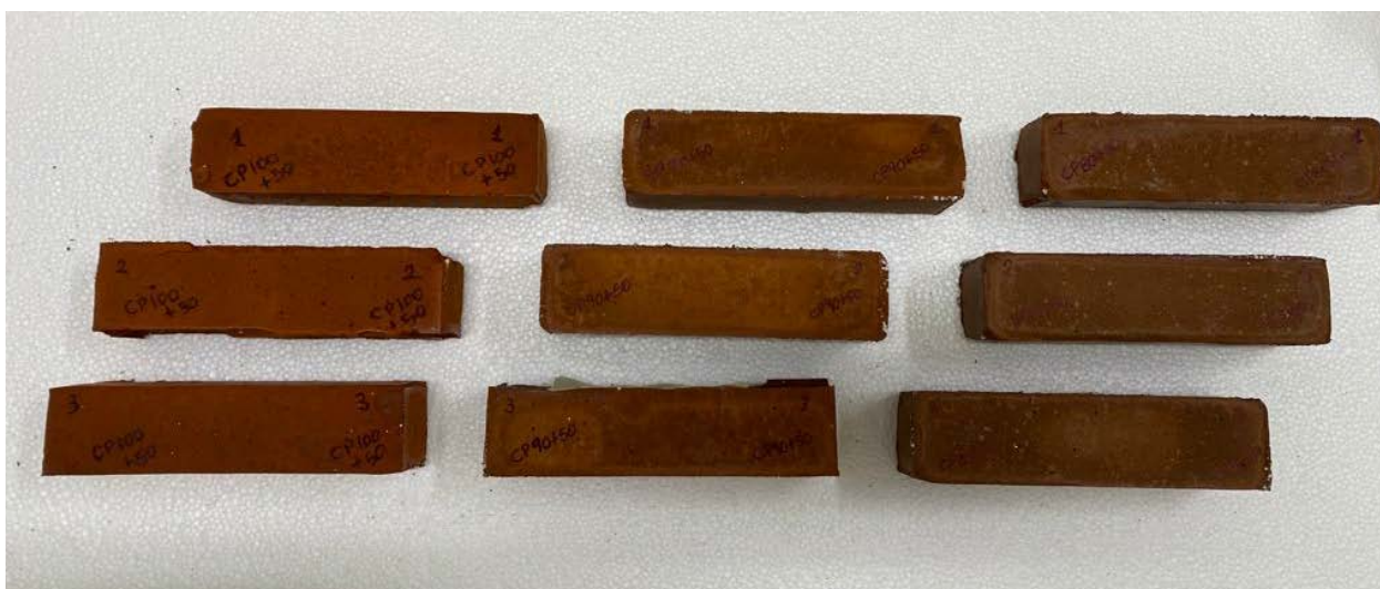
Figure n.67 - Prismatic samples of brick-based mixtures
