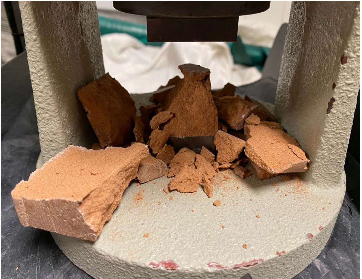
Figure 32 - Compressive strength tests on geopolymer samples
