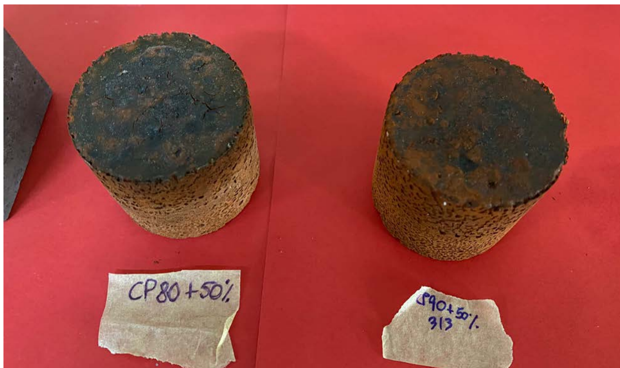
Figure n.66 - Cylindrical test pieces for mixtures with 80% and 90% brick
