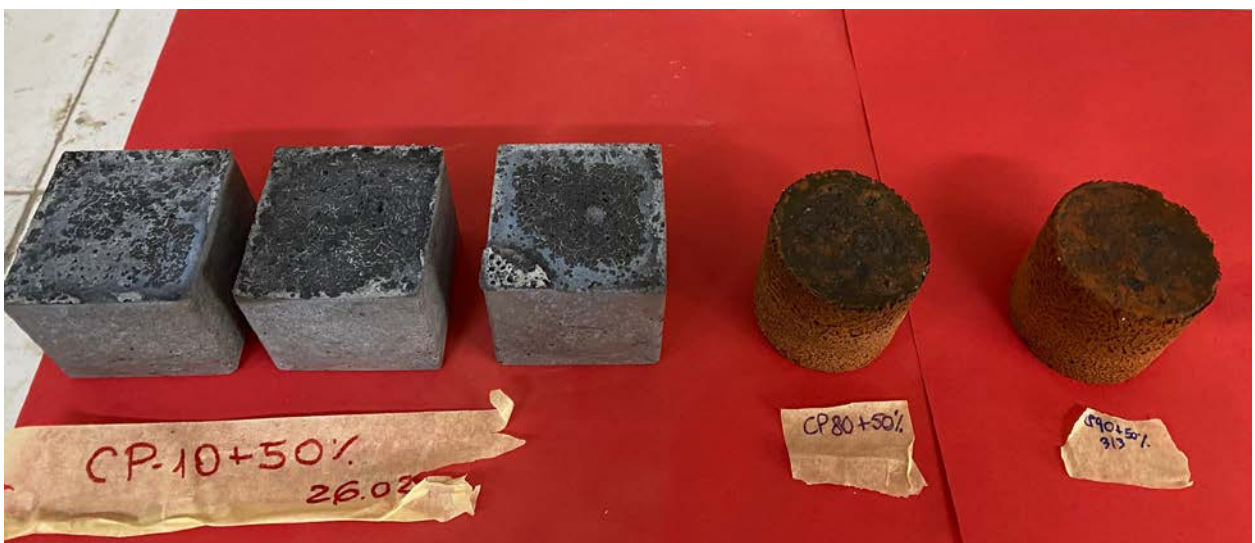
Figure n.64 - Cubic and cylindrical brick-based test specimens
