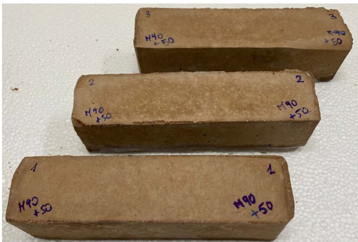
Figure n.74 - Prismatic samples of demolition mixture (percentage 90%)
