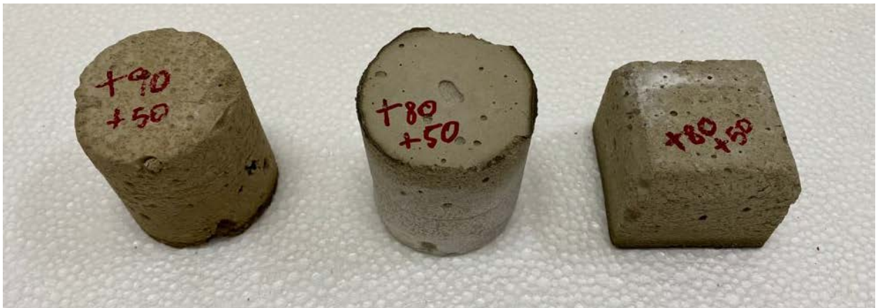
Figure n.49 - Tuff samples for physical properties characterisation tests
