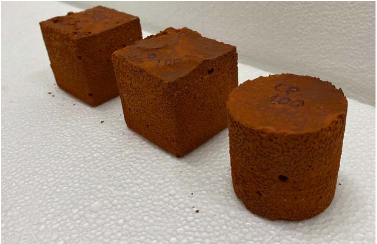
Figure n.63 - Cubic and cylindrical brick-based test specimens containing 100% demolition waste
