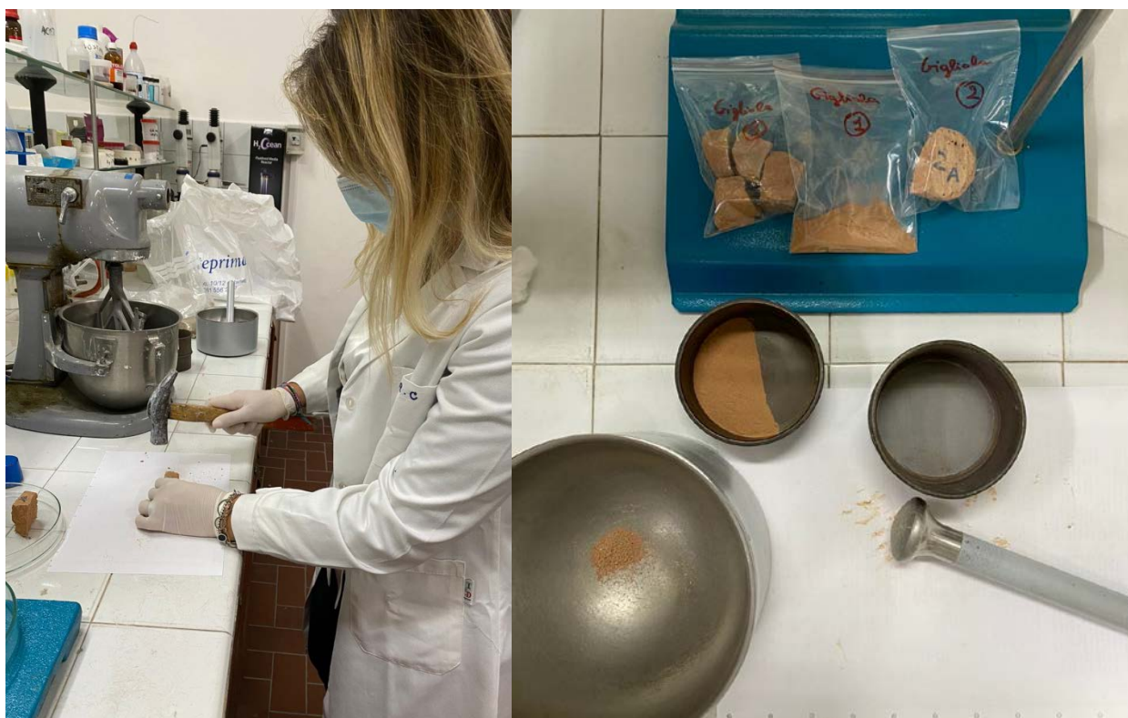
Figure n.26 - Preparation of samples for chemical and mineralogical characterisation
