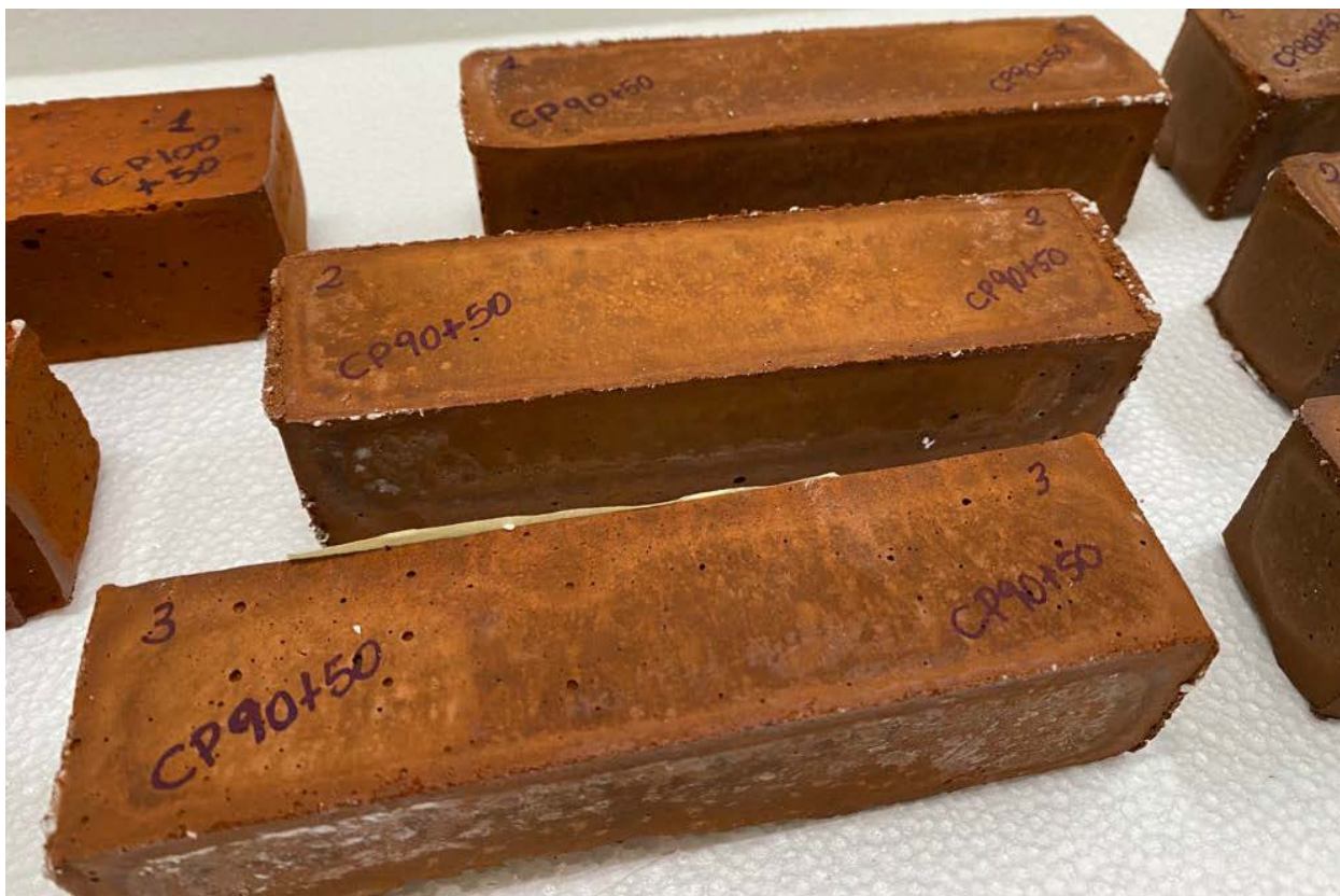
Figure n.69 - Prismatic samples for brick-based mixtures (percentage 90%)
