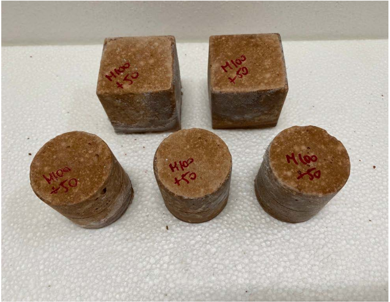
Figure n.71 - Cubic and cylindrical specimens with 100% mixed mixture
