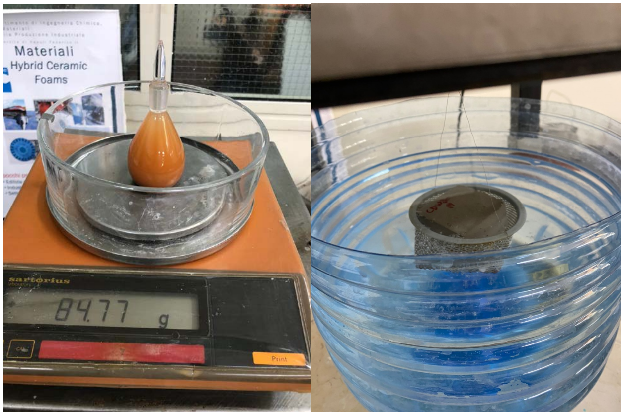
Figure n.29 - Pycnometer method and hydrostatic weighing
