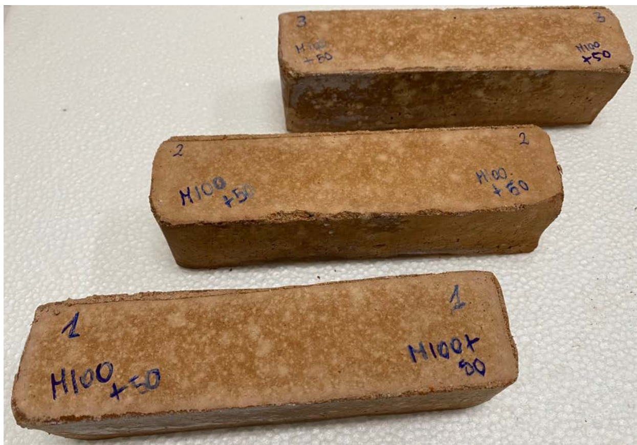
Figure n.73 - Prismatic samples of demolition mixture (percentage 100%)
