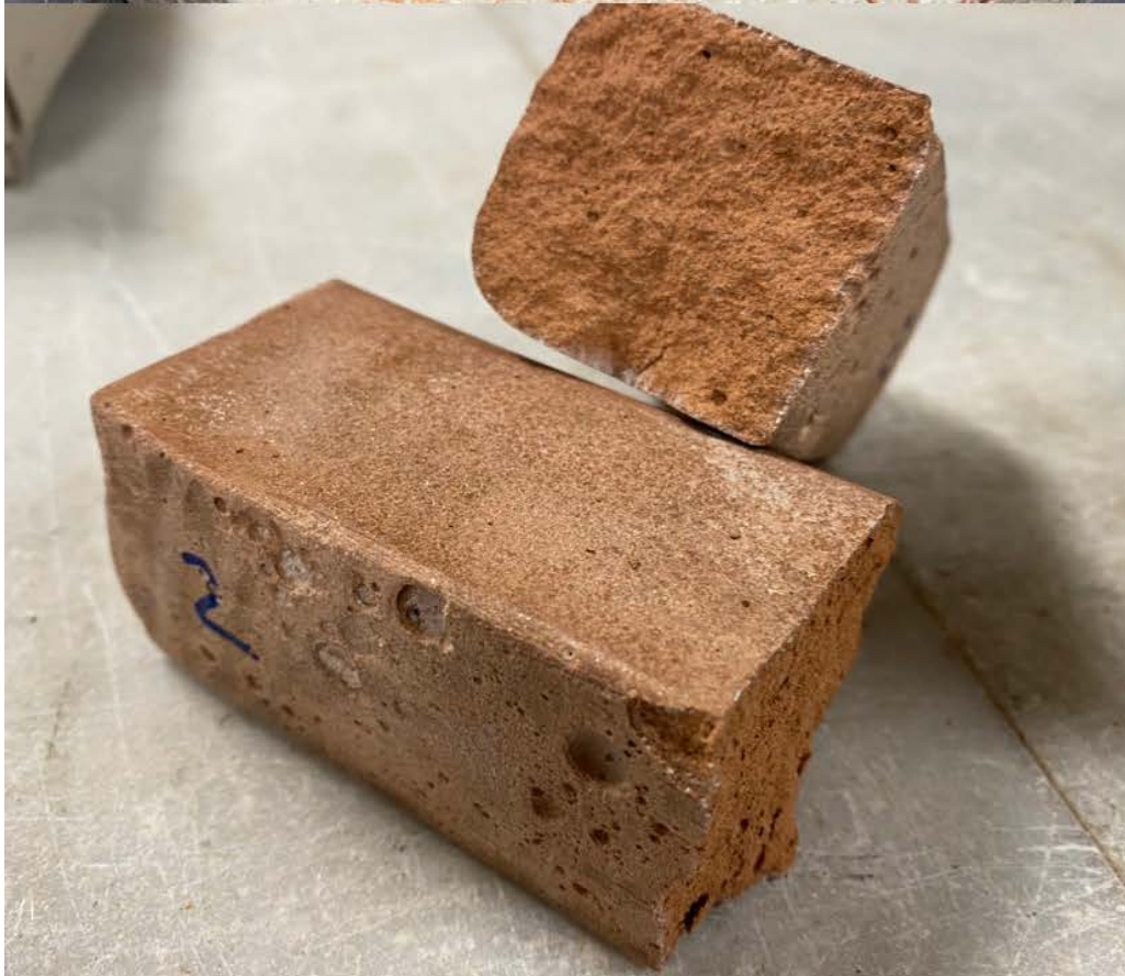
Figure n.112 - Sample tested for compressive strength and previously for flexural strength
