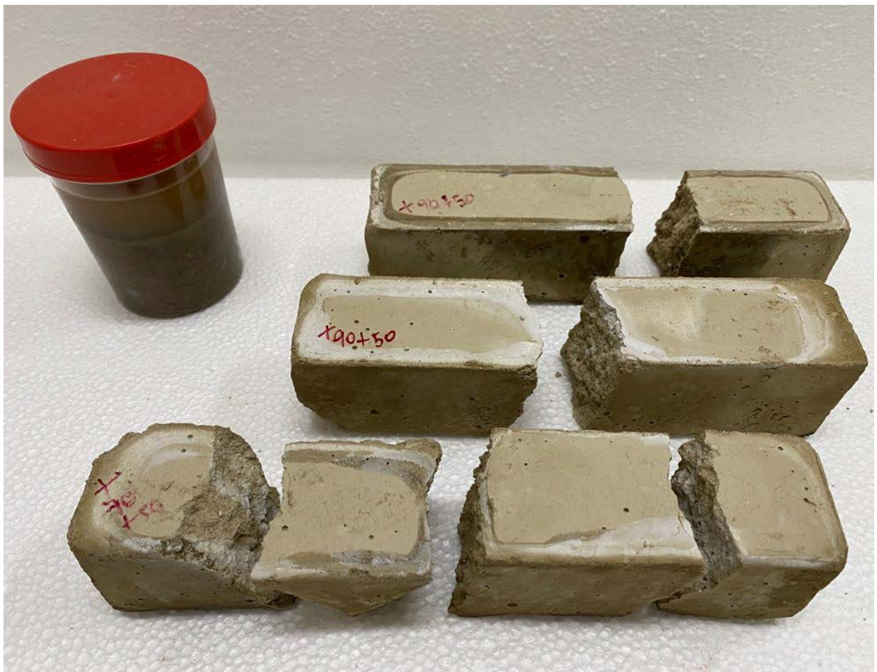
Figure n.52 - Prismatic samples of tuff according to 100% and 90% composition
