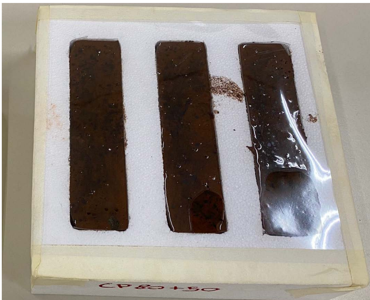
Figure n.126 - Mould with CP 80 + 50 samples produced for durability testing
