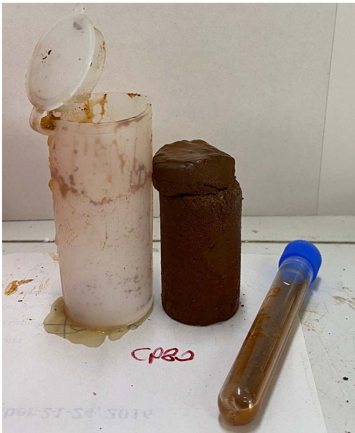
Figure n.125 – CP 80 sample after re-geopolymerisation test
