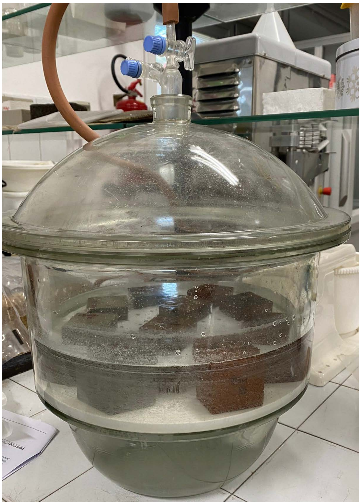
Figure n.106 - Samples subjected to the absorption test by immersion
