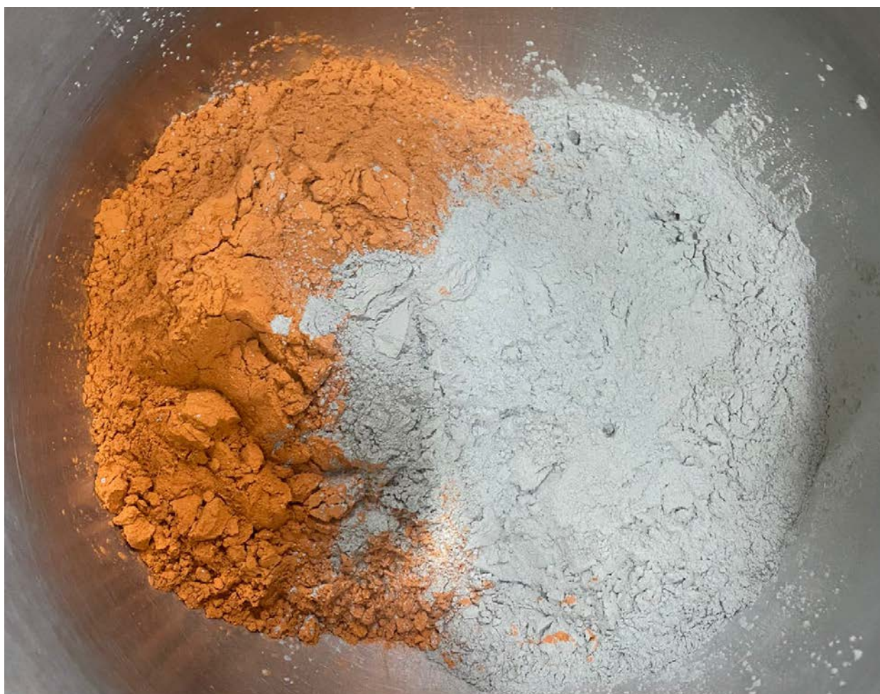
Figure n.40 - Ready-mixed materials (brick)
