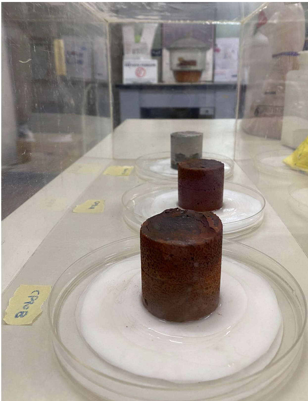
Figure n.81 - Capillary rise test (samples CP and C)
