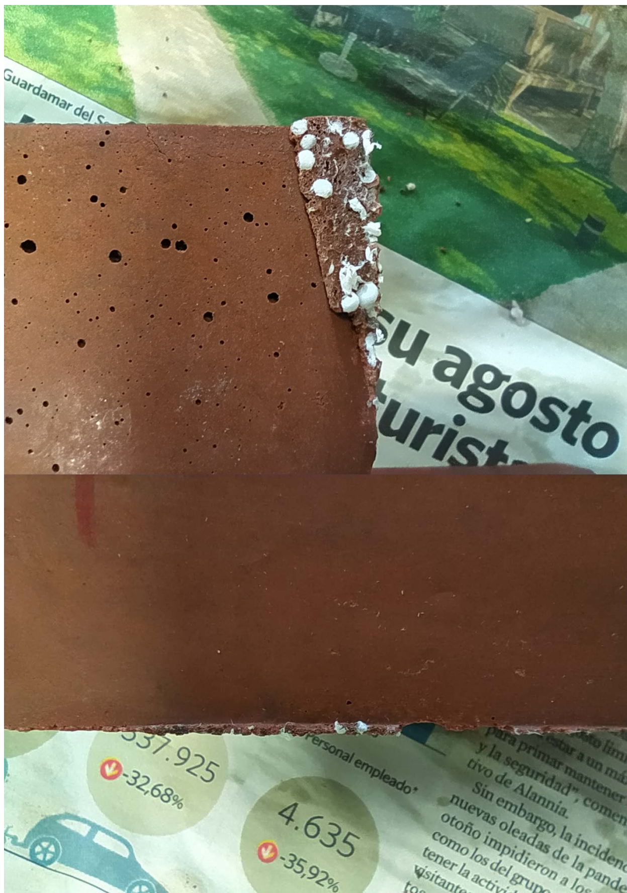
Figure n.140 - CP 80 + 50 samples detailing efflorescence after the wet chamber cycle
