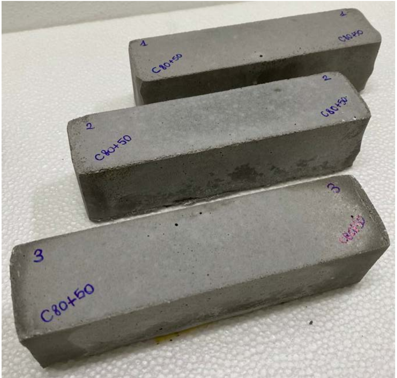
Figure n.62 - Prismatic samples of cement-based mixtures (percentage 80%)
