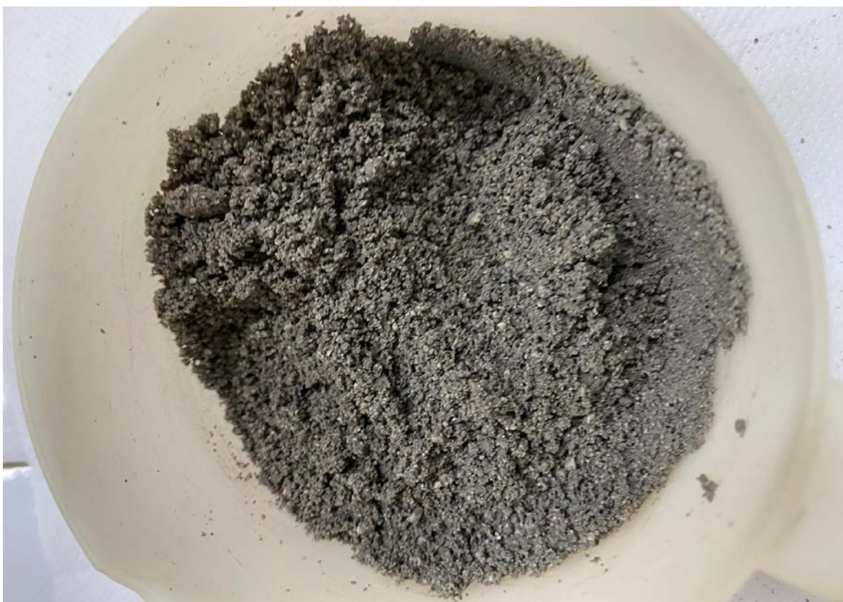
Figure n.121 - Mixing of sample C 80 for the re-geopolymerisation test
