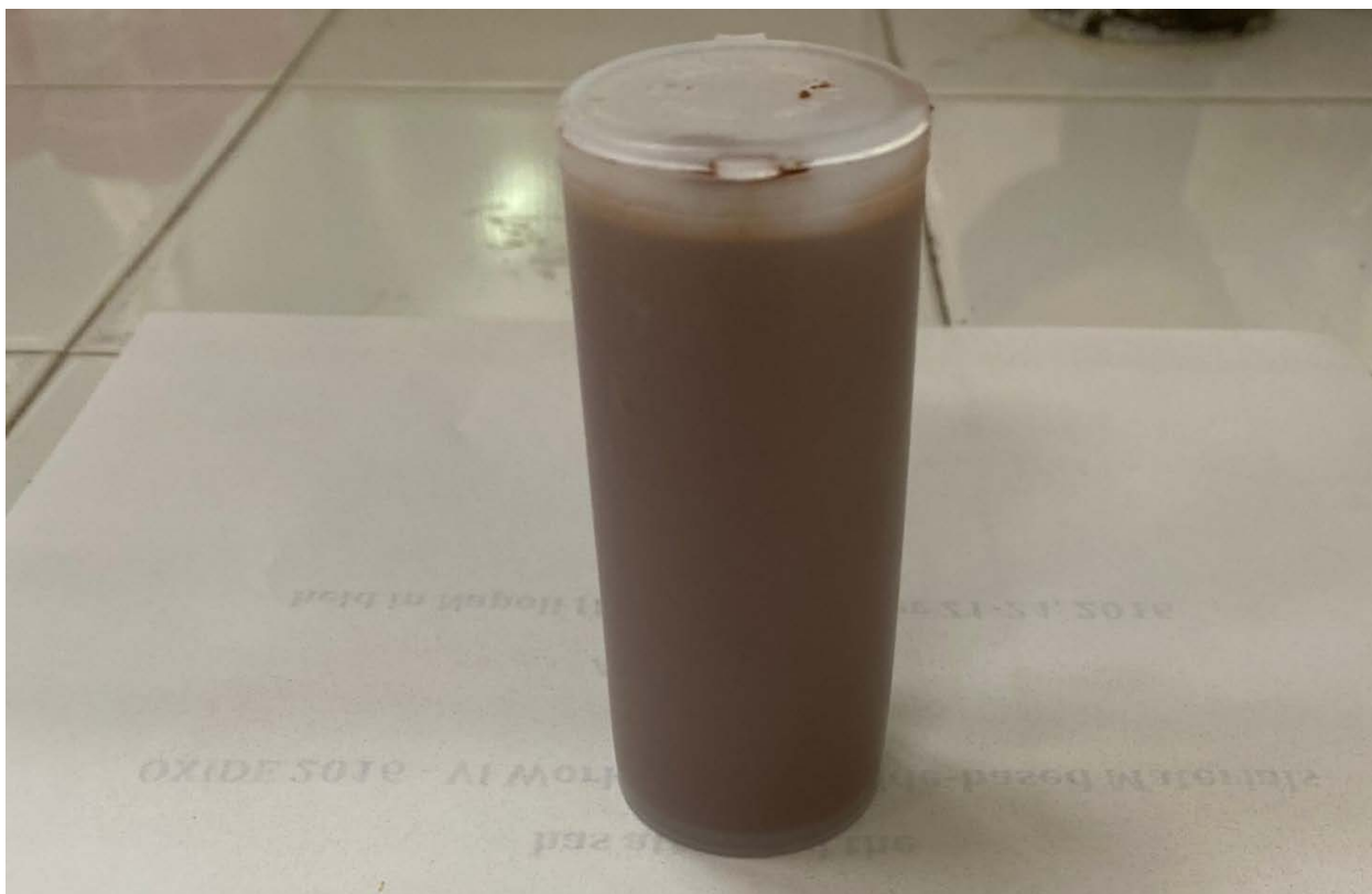
Figure n.119 - Sample CP 80 ready to be placed in the oven at 60°C for three days
