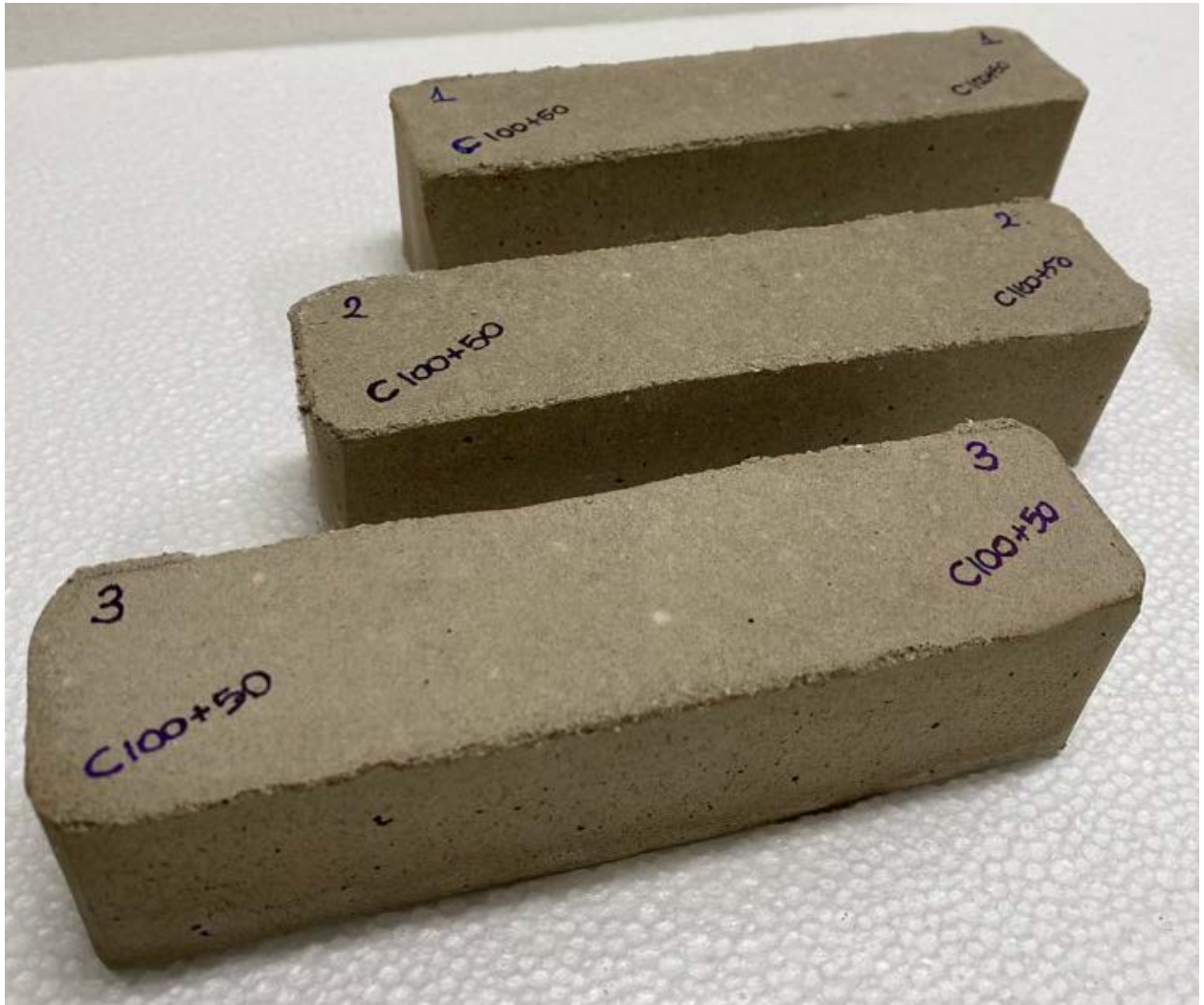
Figure n.60 - Prismatic samples of cement-based mixtures (percentage 100%)
