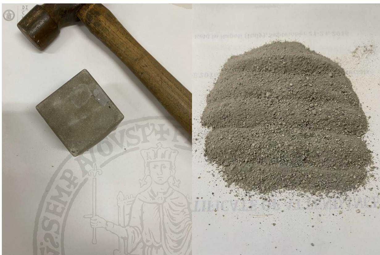
Figure n.120 - Crushing of sample C 80 for re-geopolymerisation test
