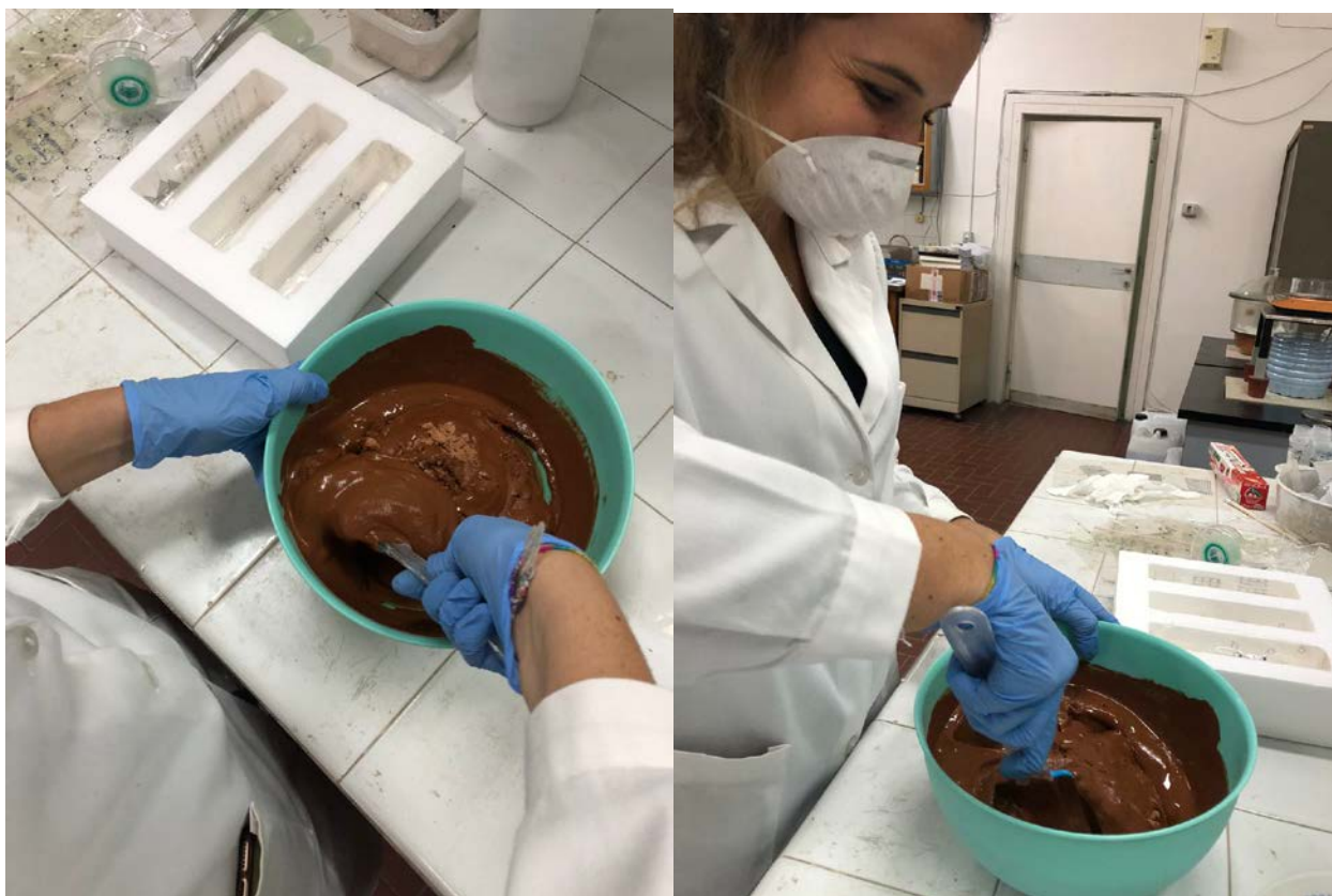
Figure n.34 - Hand production of the first 100% CP prismatic samples
