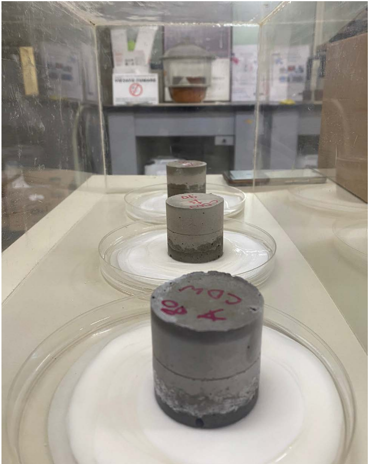
Figure n. 103 - Cement-based samples subjected to capillary absorption test
