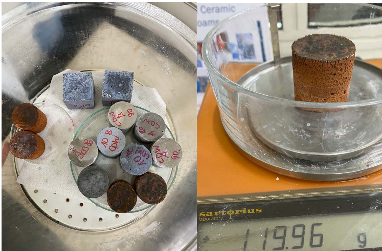
Figure n.28 - Samples ready to be weighed and subjected to the capillary rise test
