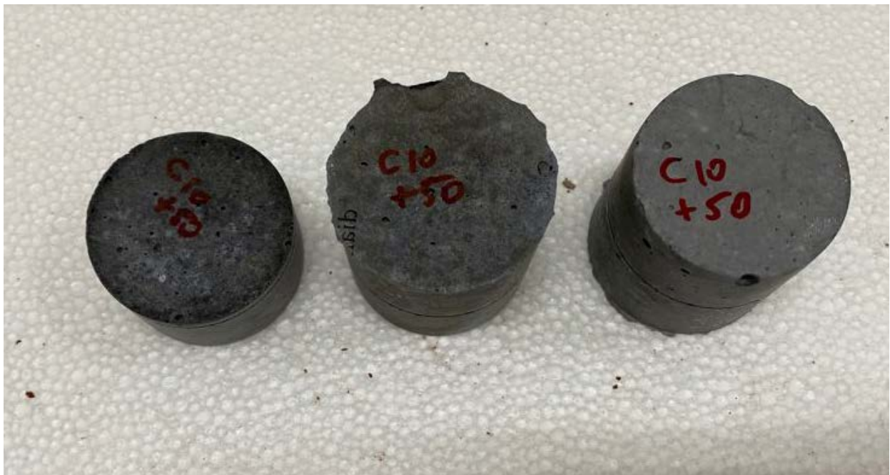
Figure n.55 - Cylindrical cement-based test specimens according to 10% composition
