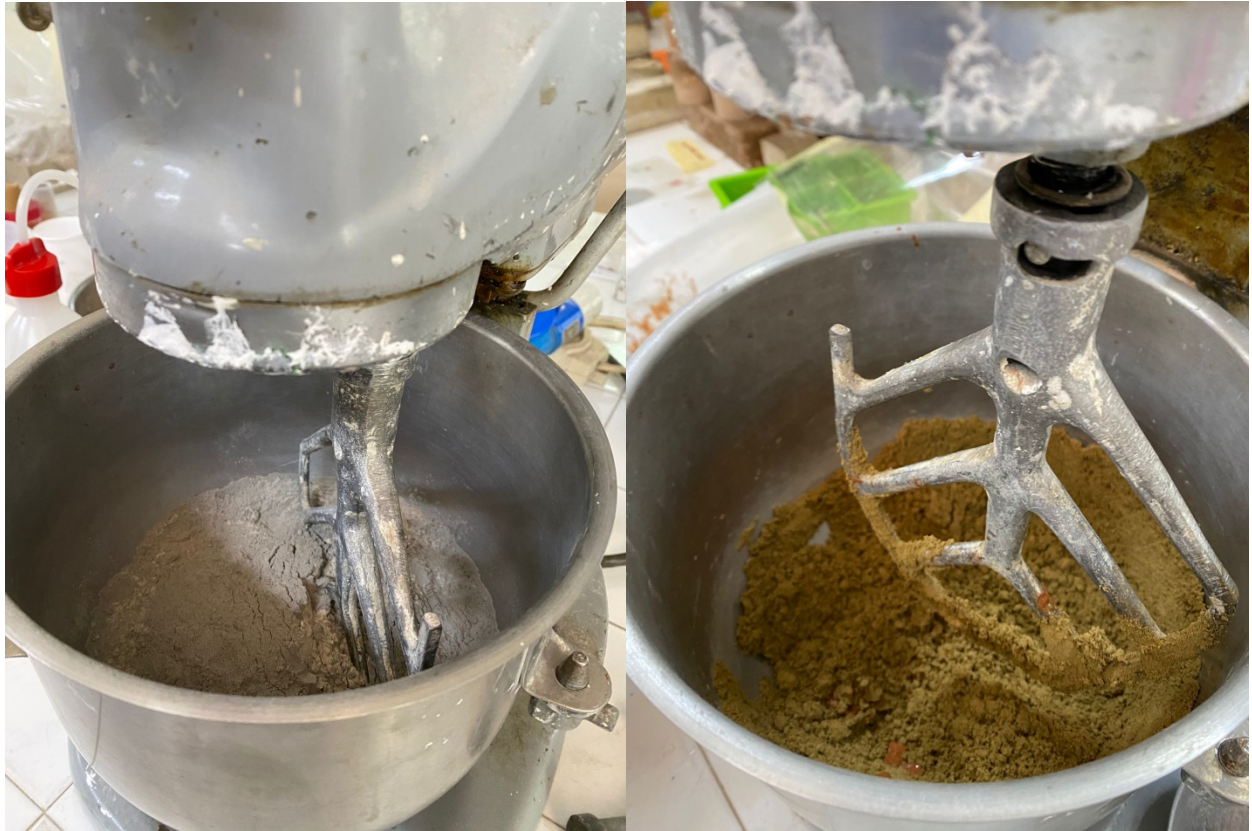
Figure n.37 - Mixing procedure in the Hobart
