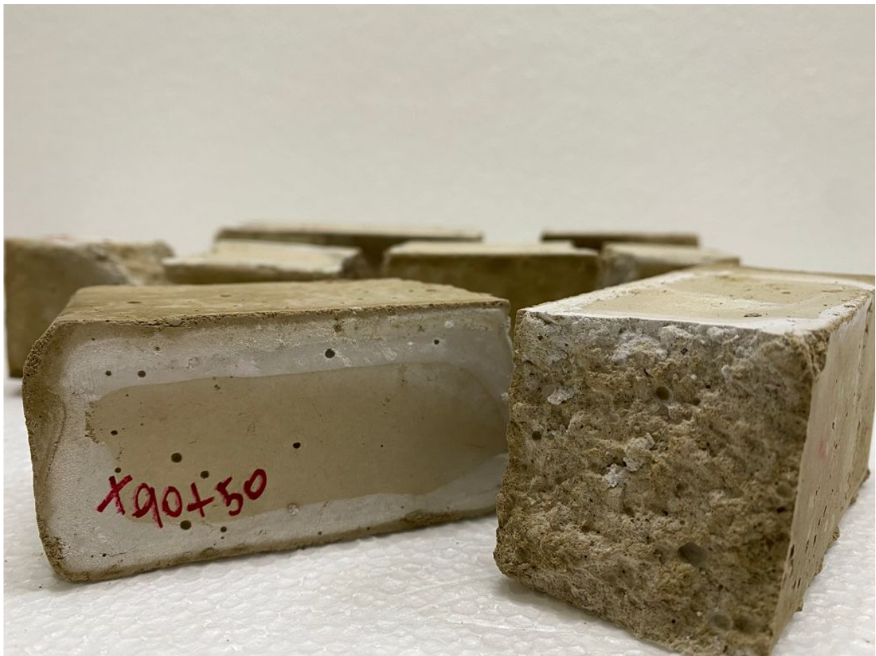
Figure n.53 - Detail of prismatic samples of 90% mixture tuff
