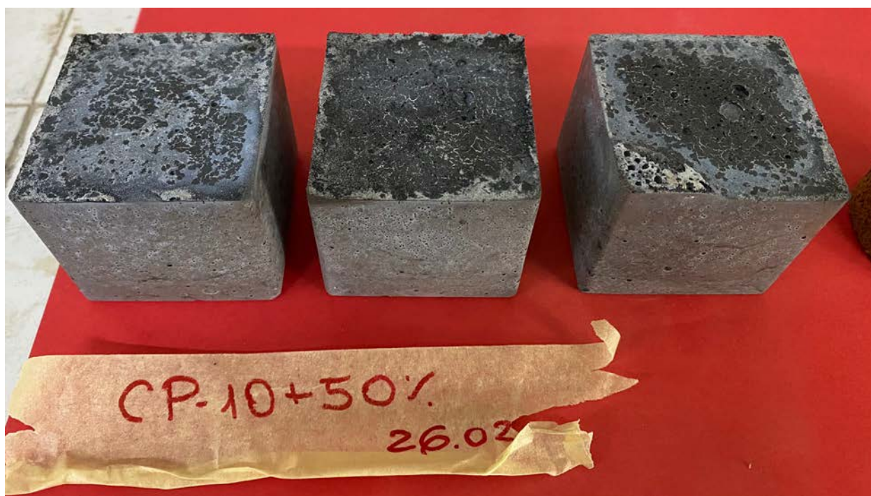
Figure n.65 - Cubic samples containing 10% demolition waste and 90% flyash
