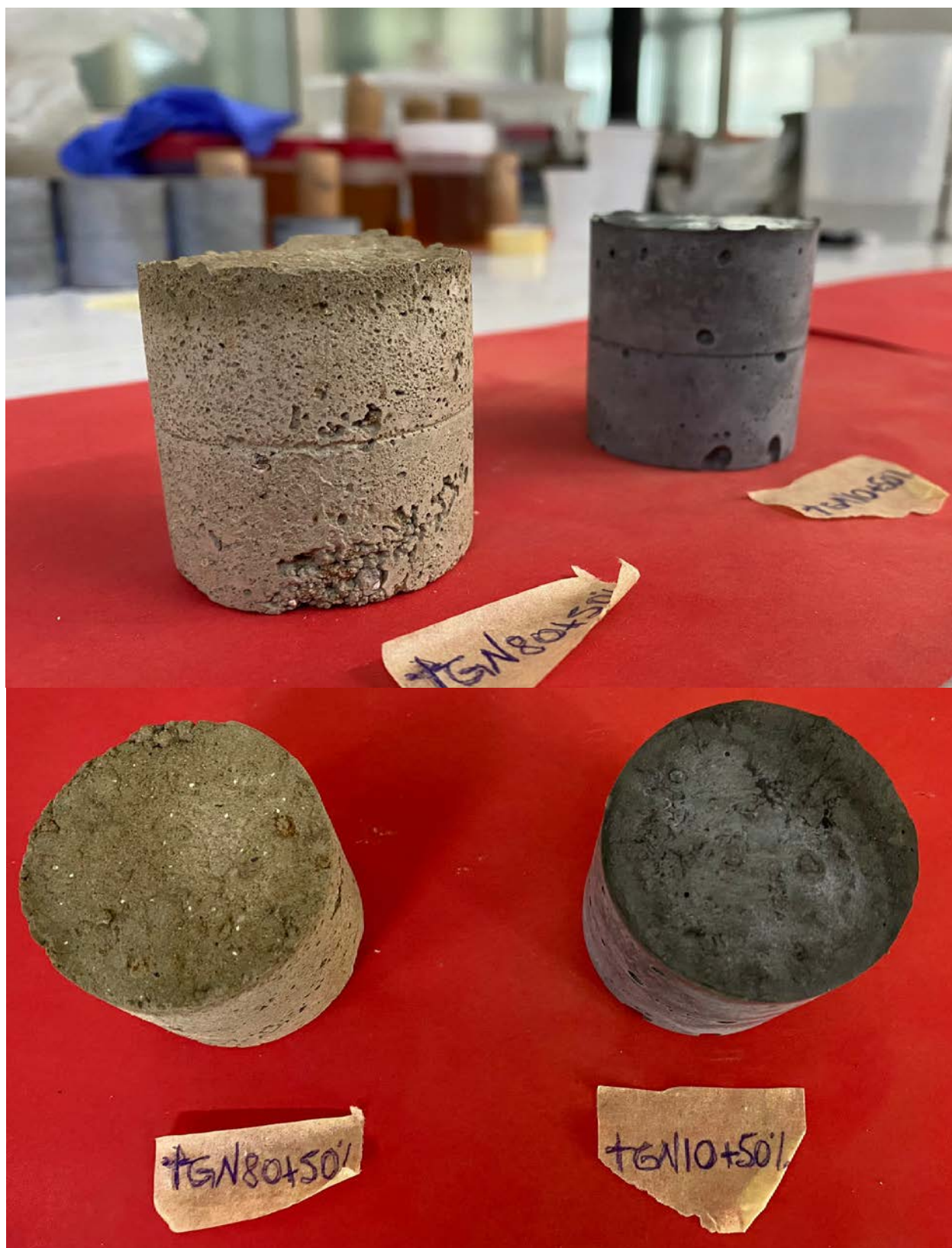
Figure n.50 - Cylindrical tuff specimens for physical properties characterisation tests
