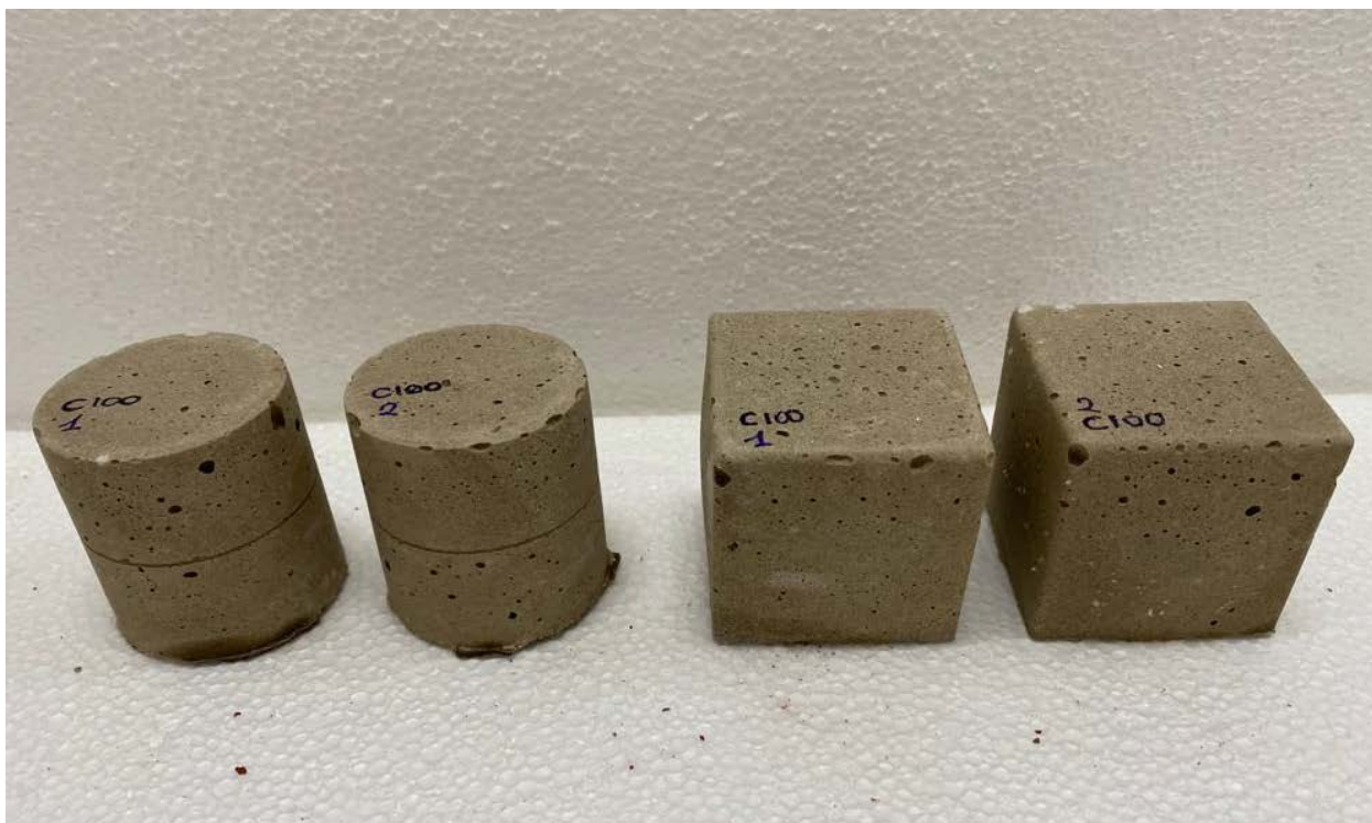
Figure n.56 - Cubic and cylindrical cement-based test specimens according to 100% composition
