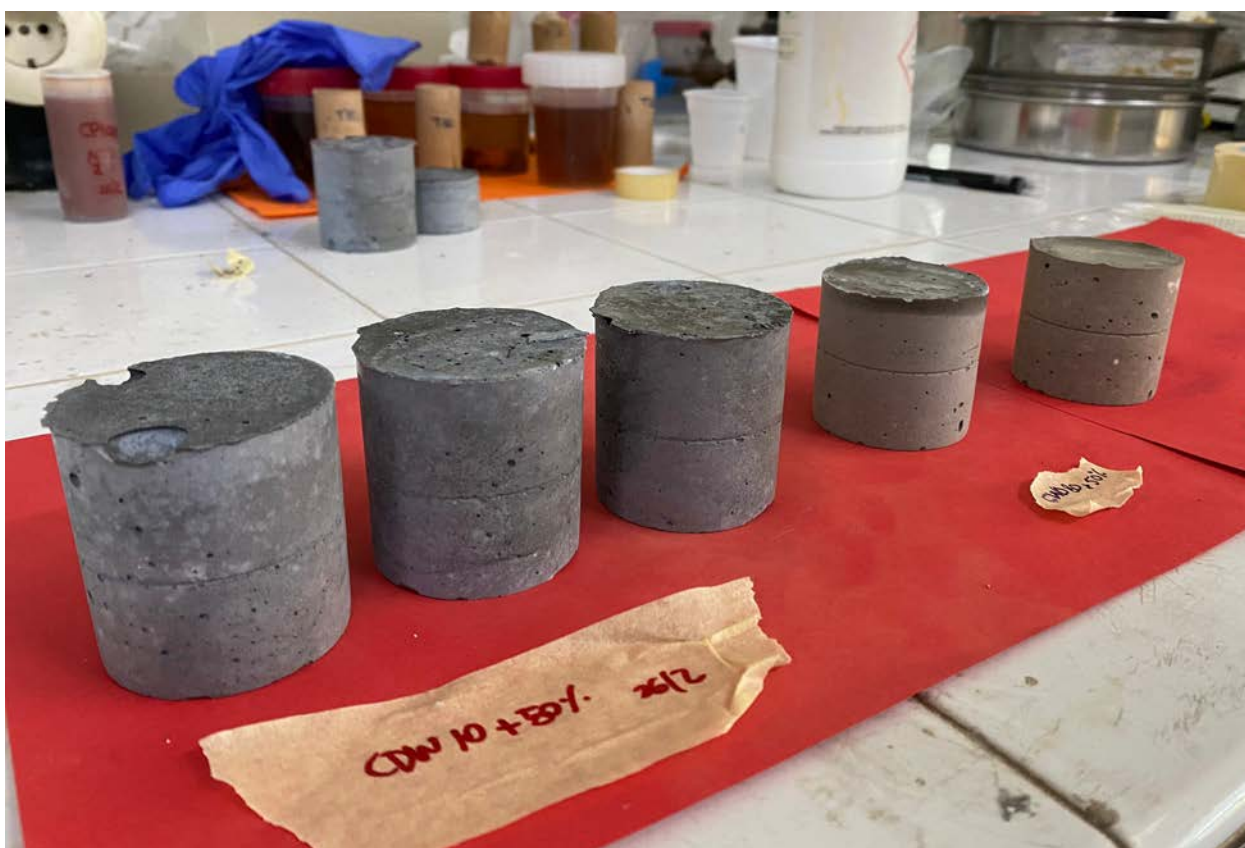
Figure n.57 - Cylindrical test pieces produced from cement residues from the demolition activity
