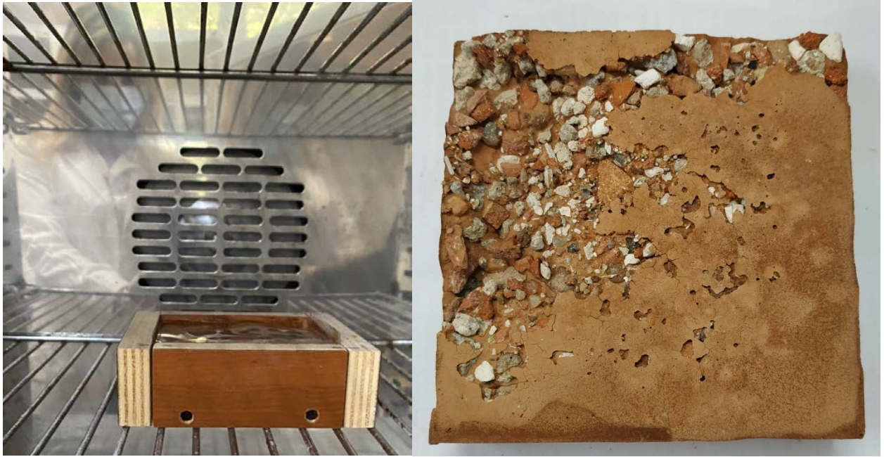
Figure n.150 – Tile in oven at 60°C and after three days
