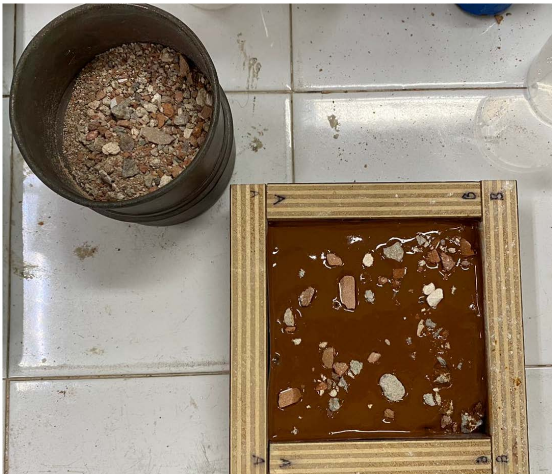
Figure n.149 - Mixture poured into the wooden mould
