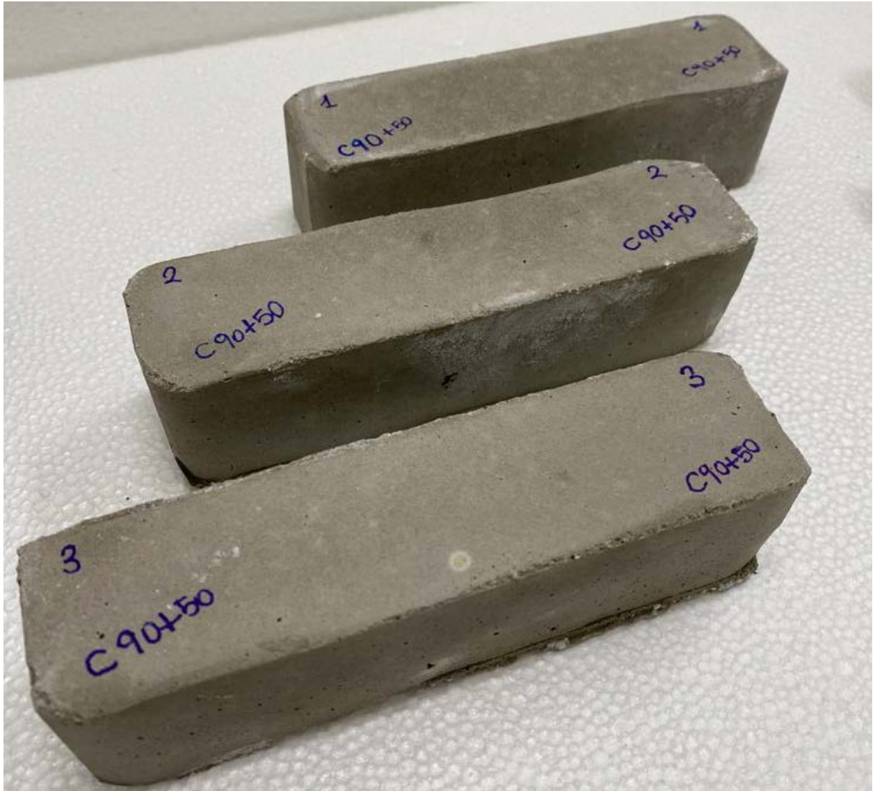
Figure n.61 - Prismatic samples of cement-based mixtures (percentage 90%)
