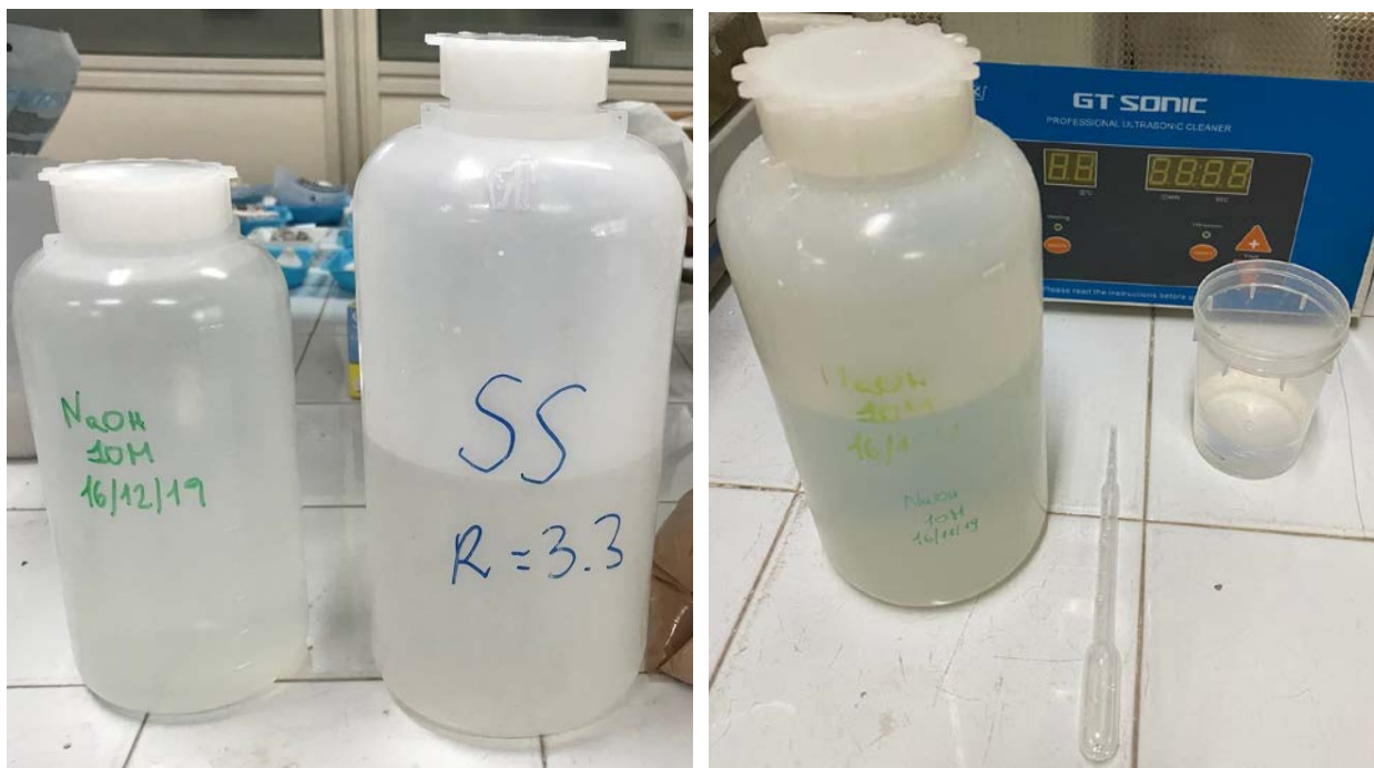
Figure n.21 - Solution of sodium silicate (SS) and 10M sodium hydroxide (NaOH)
