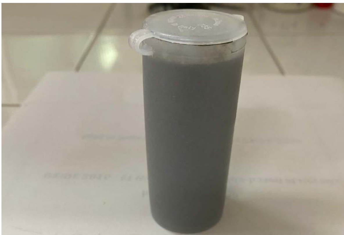
Figure n.122 - Sample C 80 ready to be placed in the oven at 60°C for three days
