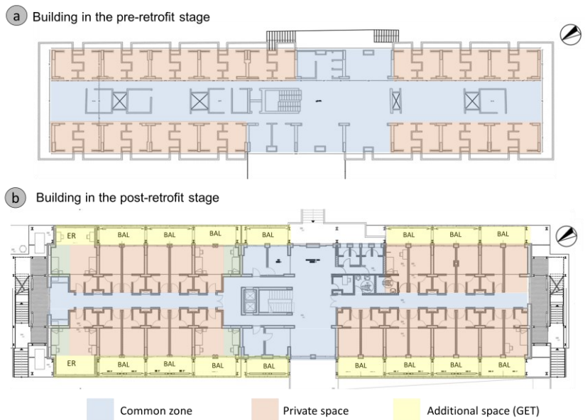
Figure 5.2 - Plans of the ground floor, before (a) and after (b) the renovation.
