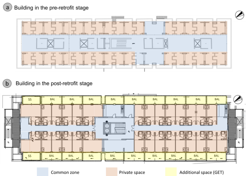
Figure 5.3 - Plans of the first floor, before (a) and after (b) the renovation
