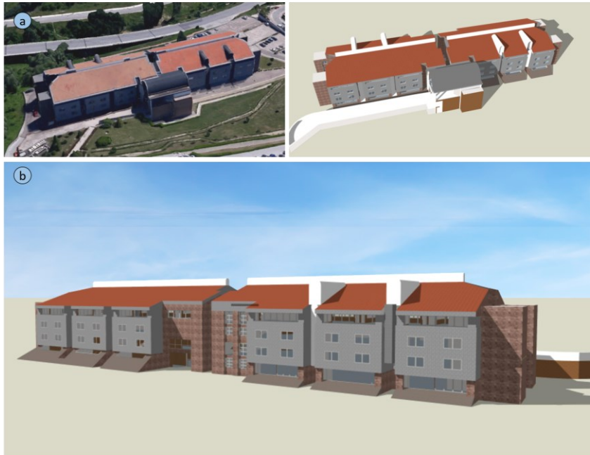
Figure 4.7 - a) real building and rendered from DesignBuilder; b) Rendering of simulation model (north-east side)
