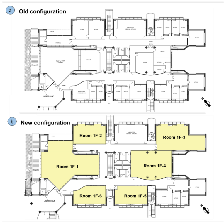
Figure 4.9 - 1 st floor of the block II: Current plan (A) and architectural renovation (B) designed for having 7 new classrooms (1 at the ground floor, 6 at the first floor)
