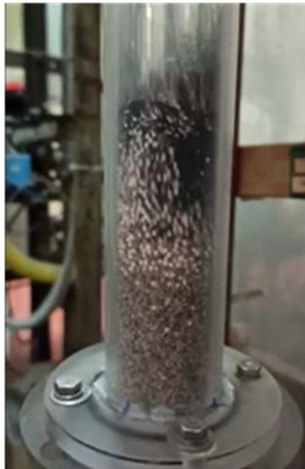
**Figure 6.10** Fluidization conditions for a bed of zeolites 3A (1.7 mm) mixed with the catalyst (0.6 mm)
