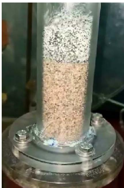
**Figure 6.10** Fluidization conditions for a bed of CaO (0.5 mm) mixed with the catalyst (0.6 mm)
