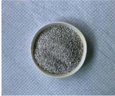
**Figure 6.1** CaO sieved in the range 400-600  $\mu\text{m}$
