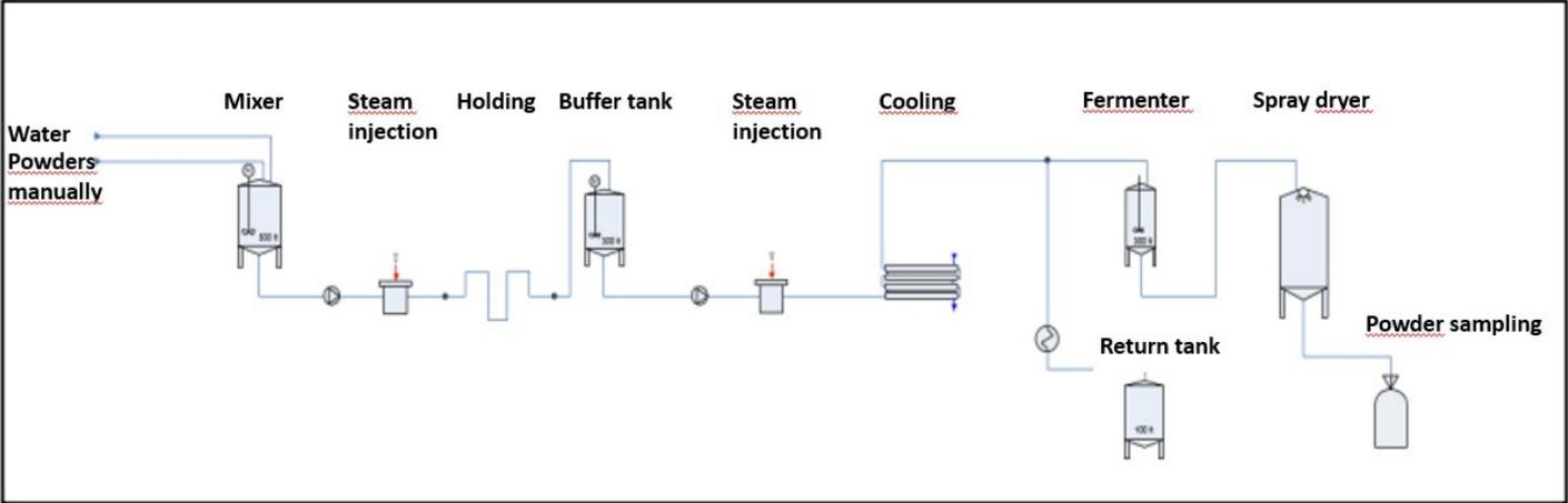
**Figure 3. Milk fermentation flowchart**
