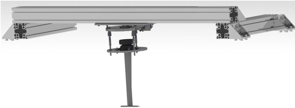
Figure 4.7: Wing assembly setup for the LMFL boundary layer wind tunnel.
