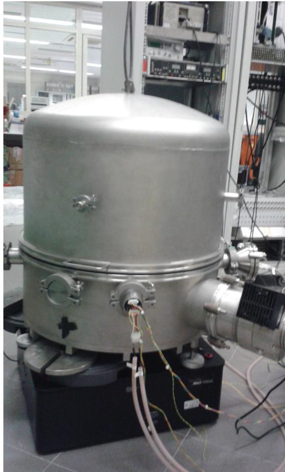
Figure 3.13: The balance installed over the Minus-K platform in the Naples laboratory
