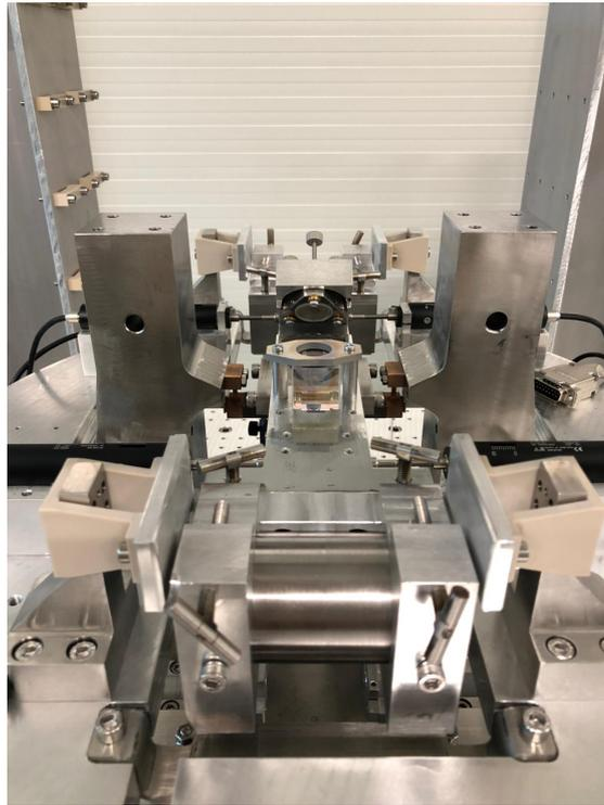
Figure 4.13: The reference arm installed on the balance
