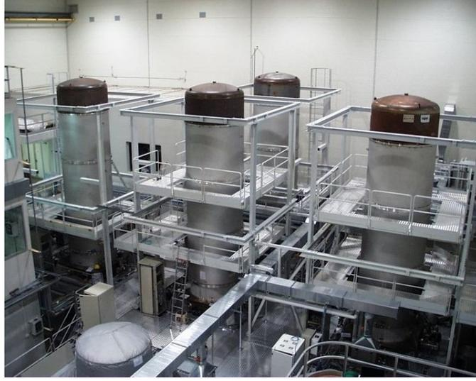
Figure 2.4: A picture of central part of Advanced Virgo. Each of the tall vacuum-chambers is hosting a Superattenuator.
