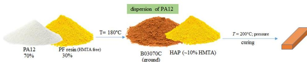
**Figure 4.30:** The schematic process used to obtain the masterbatch B0\_3070C and then the cured specimen by compression molding.
