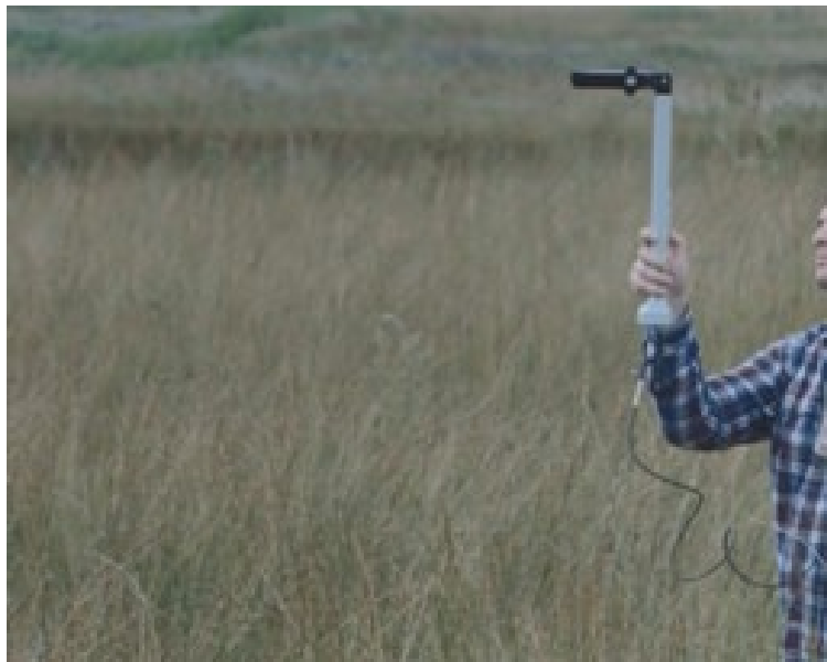
FIGURE 5.21: Indirect Leaf Area Index (LAI) estimations by LI-COR® LAI2000 Plant Canopy Analyzer
