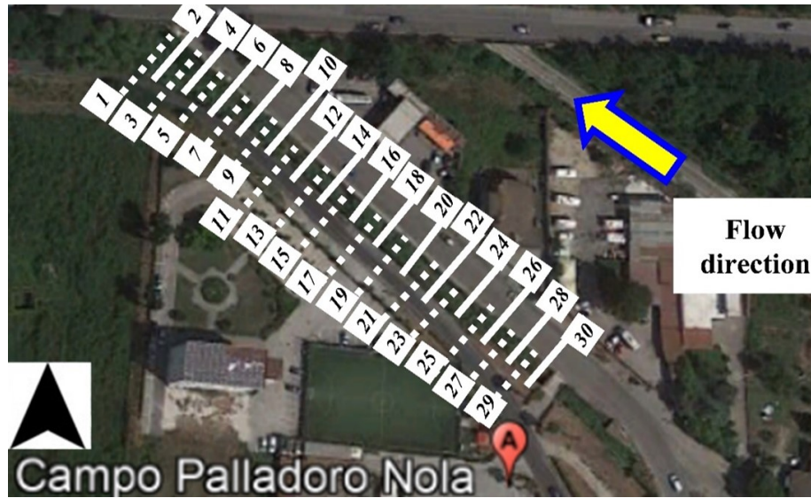
FIGURE 5.3: Aerial view of the 30 cross-sections of the vegetated drainage channel fully covered by 9 – 10m high Arundo donax , located 3.85m apart. The yellow arrow indicates the flow direction
