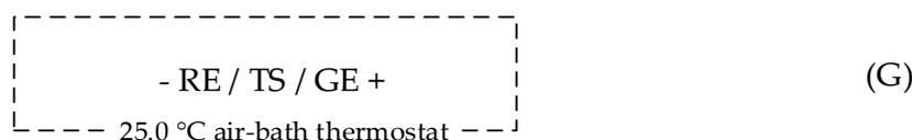
**Scheme 1.** Sketch of the potentiometric apparatus employed to prepare test solutions, TS, of accurately known pH and analytical composition. RE represents the double junction  $\text{Ag}/\text{AgCl}(\text{s})/0.1 \text{ M NaCl}/(0.1 \text{ M NaClO}_4\text{-CH}_3\text{OH}, 50/50 \text{ w/w})$  reference electrode and GE a pH indicator glass electrode
