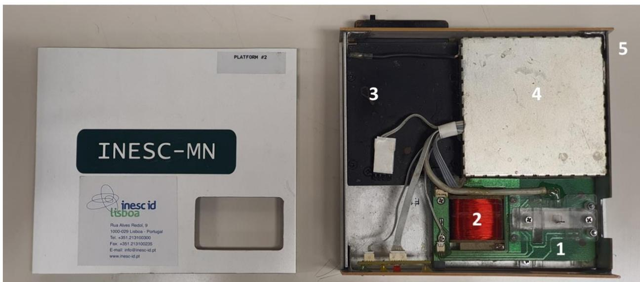
**Figure 4.8.** Detail of the biochip platform internals: 1) chip insertion site, 2) coil for magnetic drive, 3) battery, 4) box enclosing detection electronic, 5) USB port.
