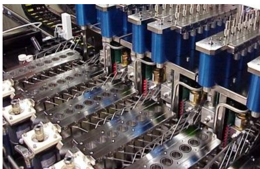
Figure 1. PPR HTE system used in this thesis work to synthesize olefin block copolymers.
