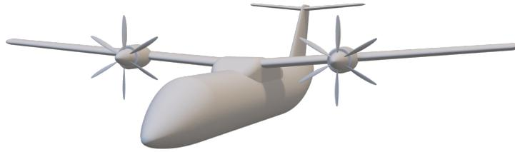
**Figure 5.1:** Conventional regional turboprop designed for the PROSIB project.
